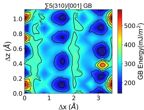
Fig. 1 Calculated  $\gamma$ -surface for a  $\Sigma 5(310)/[001]$  GB.
