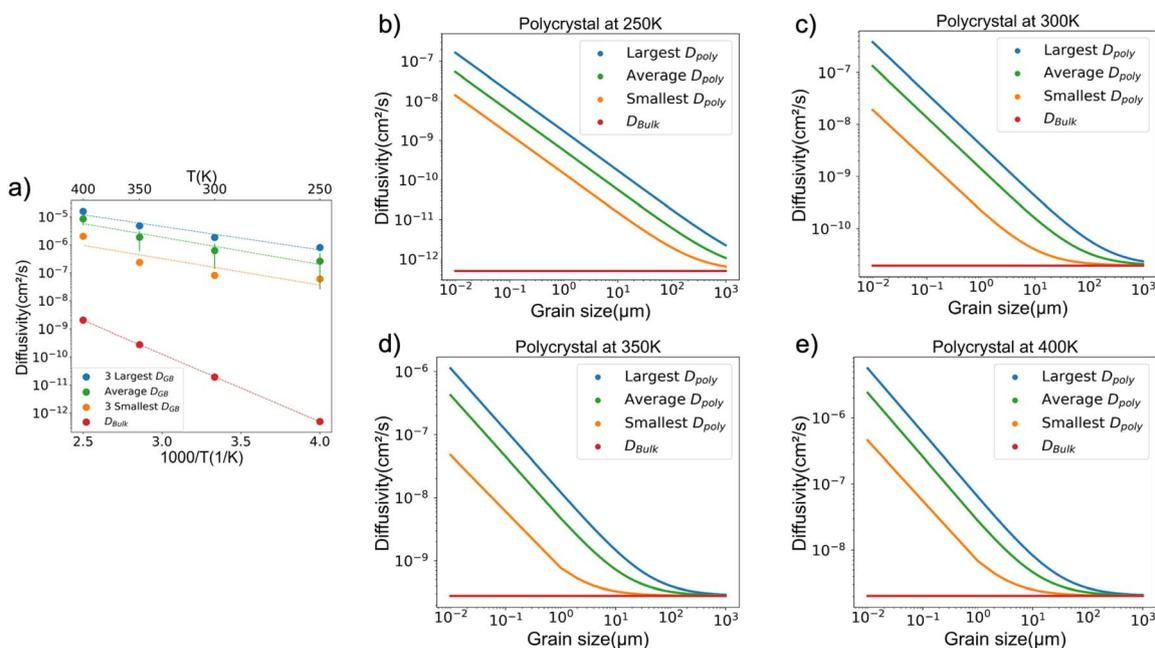
Fig. 6 (a) The average of the 3 fastest, 3 slowest, and overall average GB diffusivities vs. inverse temperature. Polycrystalline diffusivity (eqn (6)) as a function of grain size at (b) 250 K (c) 300 K (d) 350 K (e) 400 K. Here “Largest,” “Smallest,” etc. refers to the range of D<sub>GB</sub> shown in panel (a).
