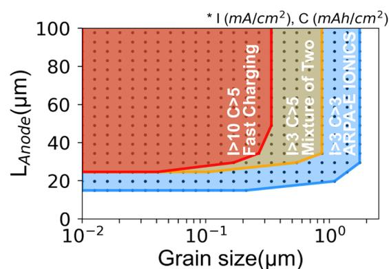
Fig. 9 Design guidelines for capacity ( $C$ ) and current density ( $I$ ) based on anode thickness and grain size. Conditions that satisfy the fast-charging goal ( $I > 10$   $C > 5$ ) are shown in red, those that satisfy the ARPA-E ionic goal ( $I > 3$   $C > 3$ ) are shown in blue, and those that satisfy a mixture ( $I > 3$   $C > 5$ ) are orange.
