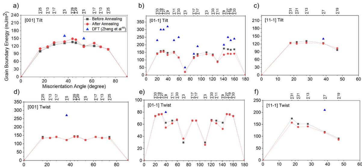
Fig. 4 GB energy before/after annealing as a function of misorientation angle. (a) [001] tilt (b) [01-1] tilt (c) [11-1] tilt (d) [001] twist (e) [01-1] twist (f) [11-1] twist rotation axis. The  $\Sigma$ -values of the coincidence site lattice are listed at the top axis of each plot. Recent energies calculated from DFT are shown for comparison.<sup>42</sup>
