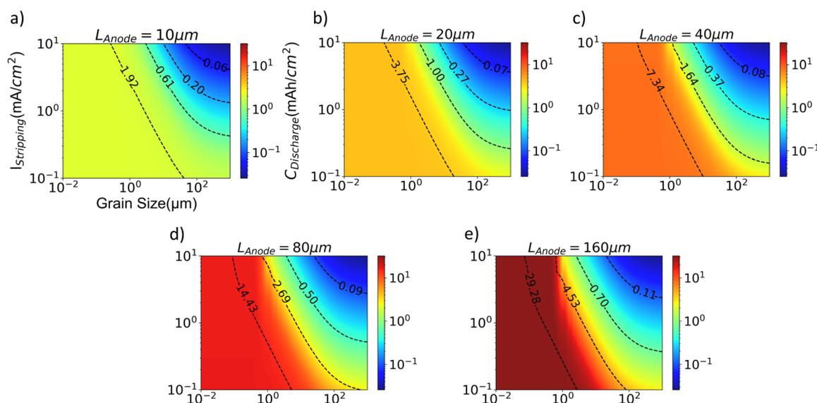
Fig. 8 Maximum discharge capacity as a function of stripping current and grain size for Li anode thicknesses of (a) 10  $\mu\text{m}$ , (b) 20  $\mu\text{m}$ , (c) 40  $\mu\text{m}$ , (d) 80  $\mu\text{m}$ , and (e) 160  $\mu\text{m}$ .
