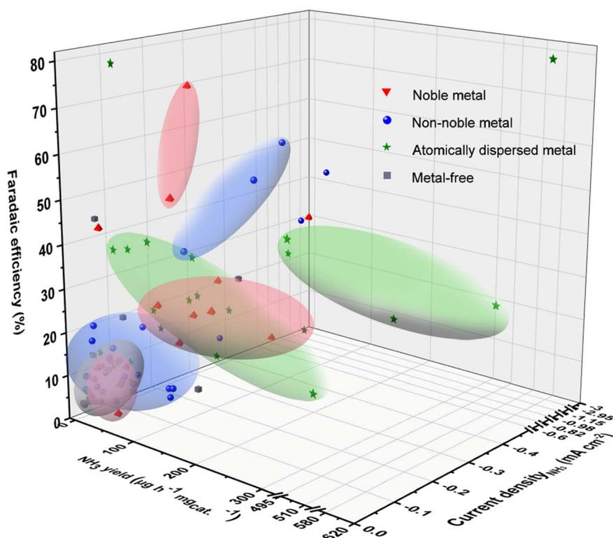
Fig. 2 Summary about the experimental performances ( $NH_3$  yield, FE, and current density ascribed to  $NH_3$ ) of reported eNRR catalysts. The specific performances are shown in Table 1.
