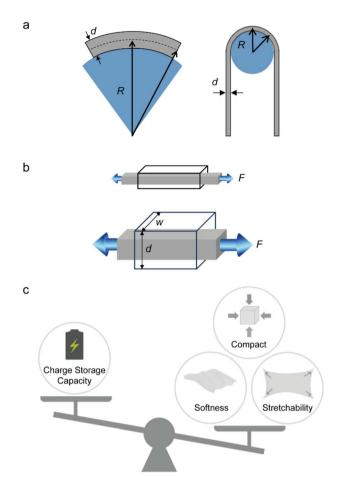
Fig. 2 Illustrations of a rectangular shaped beam that is (a) bent and (b) stretched, where d is the thickness, R is the bending radius, and F is the force needed to deform the object. (c) The trade-off between the charge storage capacity and the mechanical properties of the battery.
