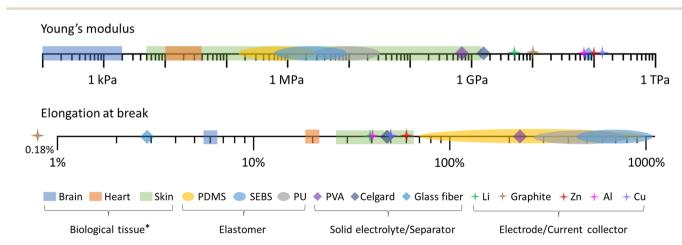
Fig. 3 Young's modulus (top) and elongation at break (bottom) of conventional battery materials and elastomers in comparison with representative biological tissues (\*maximum tensile strain in biomechanical environment).9,54-59
