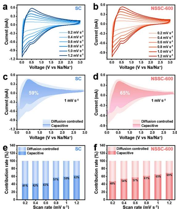
Fig. 6 CV curves of (a) SC and (b) NSSC-600 at the scan rates from 0.2 to 1.2  $\text{mV s}^{-1}$ . Capacitive contribution area of (c) SC and (d) NSSC-600 at 1.0  $\text{mV s}^{-1}$ . Capacitive contribution ratios of (e) SC and (f) NSSC-600 at the scan rates from 0.2 to 1.2  $\text{mV s}^{-1}$ .
