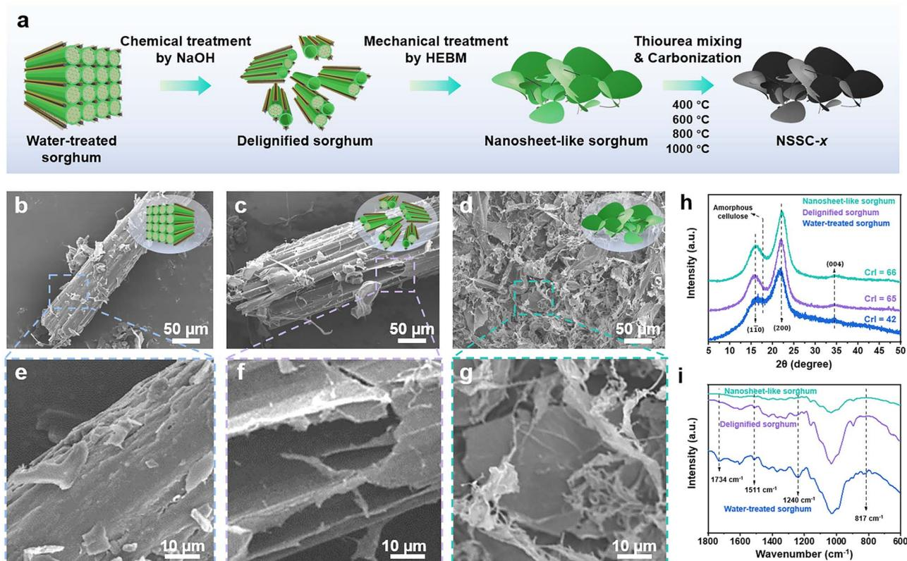
**Fig. 1** (a) Description of the synthesis of NSSC-*x*. FESEM images of (b) water-treated sorghum, (c) delignified sorghum, and (d) nanosheet-like sorghum. Enlarged FESEM images of (e) water-treated sorghum, (f) delignified sorghum, and (g) nanosheet-like sorghum. (h) XRD and (i) ATR-FTIR spectra of sorghum samples at each stage of treatment.
