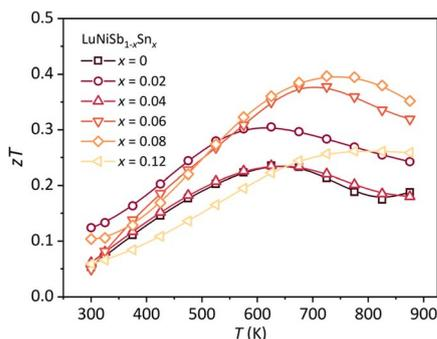
Fig. 7 Temperature dependence of  $zT$  for  $\text{LuNiSb}_{1-x}\text{Sn}_x$ .
