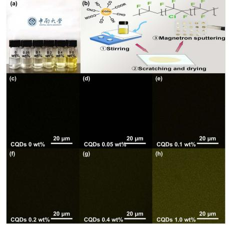
Fig. 2 (a) Digital images of CQDs/P(VDF-TrFE-CTFE) solutions with different CQD content. (b) The scheme of the nanocomposite fabrication. (c-h) The fluorescence images of the nanocomposites recorded by LSCM.
