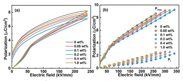
Fig. 7 (a) The P-E loops at 240 kV mm<sup>-1</sup> and (b) the maximum polarization and remanent polarization at different electric fields of the samples with different CQD content.
