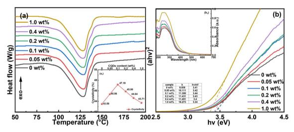
Fig. 6 (a) The DSC curves. (b) The Tauc plot. (a<sub>1</sub>) The crystallinity. (b<sub>1</sub>) The UV-vis absorption spectra of the samples with different CQD content.
