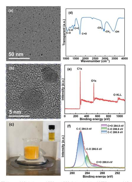
Fig. 1 (a and b) High-res TEM images. (c) Digital images of CQDs and CQDs/ethanol solution. (d) FTIR spectrum. (e) Survey XPS spectrum. (f) C 1s high-resolution XPS spectra of CQDs.
