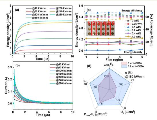
Fig. 8 (a) The  $W_d$  as a function of time and (b) pulsed overdamped discharge behaviour of the sample with CQD content of 0.1 wt% at various electric fields. (c) The film stability at 160 kV mm<sup>-1</sup> of the samples with different CQD content and (d) the comparison between the pristine polymer film and the sample with CQD content of 0.1 wt%.
