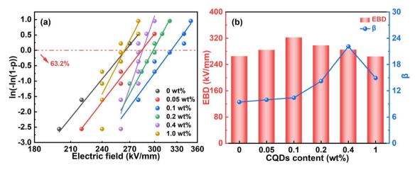
Fig. 4 (a) The Weibull distribution. (b) The corresponding EBD and shape parameters of the samples with different CQD loadings.
