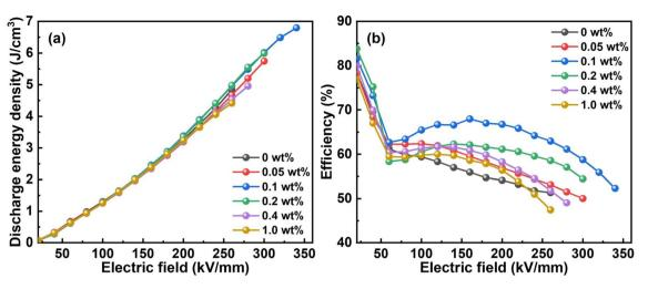
Fig. 5 (a) The discharge energy density and (b) energy efficiency of the samples with different CQDs content.
