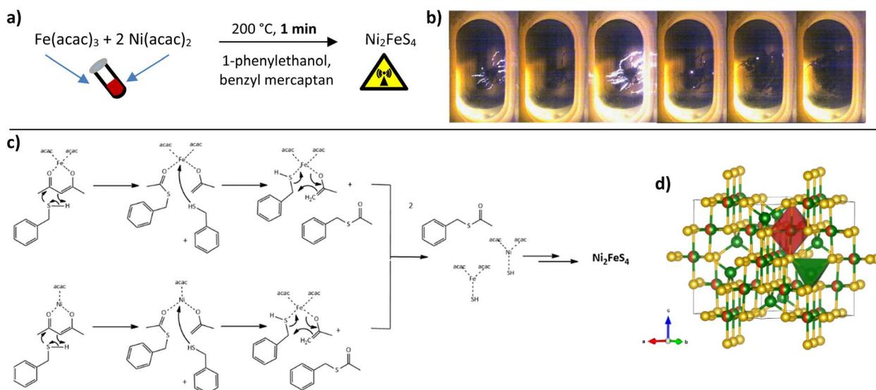
Fig. 1 General reaction equation for the formation of  $\text{Ni}_2\text{FeS}_4$  (a), photographs of observed light flashes and nanosheet formation (b), reaction sequence based on a nucleophilic attack of benzyl mercaptan similar to what was reported for alcohols (c) and crystal structure (d).
