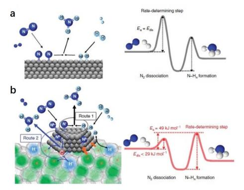
Fig. 7 Reaction mechanism and energy diagram for NH<sub>3</sub> synthesis on (a) conventional catalyst and (b) Ru/C12A7:e<sup>-</sup> catalyst. Copyright 2015, Springer Nature.
