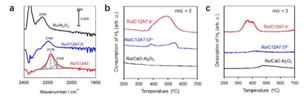
Fig. 6 (a) Difference FT-IR spectra of  $N_2$  adsorbed on  $Ru/Al_2O_3$ ,  $Ru/C12A7:O^2^-$ , and  $Ru/C12A7:e^-$  at -170 °C. Copyright 2012, Springer Nature. (b)  $H_2$ -TPA and (c) Ar-TPD profiles of  $Ru/CaO \cdot Al_2O_3$ ,  $Ru/C12A7:O^2^-$ , and  $Ru/C12A7:e^-$ . Copyright 2015, Springer Nature.
