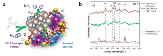
Fig. 24 (a) Schematic diagram of the ammonia synthesis reaction over Ru/C12A7:e $^-$ . (b) The inelastic neutron-scattering spectra of Ru/C12A7:e $^-$  collected at 5 K after exposure to (1) 0.1 MPa 3:1 H<sub>2</sub>: N<sub>2</sub> mixture, (2) vacuum, (3) 0.1 MPa H<sub>2</sub>, and (4) 5 cycles of 0.1 MPa N<sub>2</sub> at 673 K. Copyright 2020, American Chemical Society.
