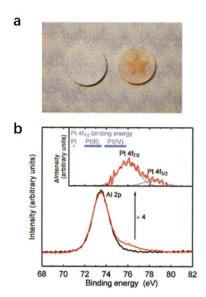
Fig. 17 (a) Photographs of the C12A7 ceramics sintered in wet air (left) and dry oxygen (right). (b) XPS spectra for the brown-colored area (red line) and the uncolored area (black line). Inset is the difference between the two spectra. Copyright 2002, American Chemical Society.
