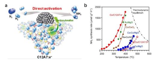
Fig. 8 (a) Reaction mechanism for NH<sub>3</sub> synthesis on Co/C12A7:e<sup>-</sup> catalyst. (b) Temperature dependence of NH<sub>3</sub> synthesis rate for the supported Co catalysts. Reaction conditions: WHSV, 18 000 mL  $g^{-1}$   $h^{-1}$ ; pressure, 0.1 MPa. Copyright 2019, American Chemical Society.
