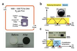
Fig. 2 Synthesis processes for C12A7 electride under a reducing atmosphere. (a) Schematic illustration of CO/CO2 reduction treatment and image of the obtained dark green electride disk. Copyright 2007, Springer Nature. Melt-solidification (b) and glass-ceramic (c) processes. Copyright 2005, American Chemical Society.
