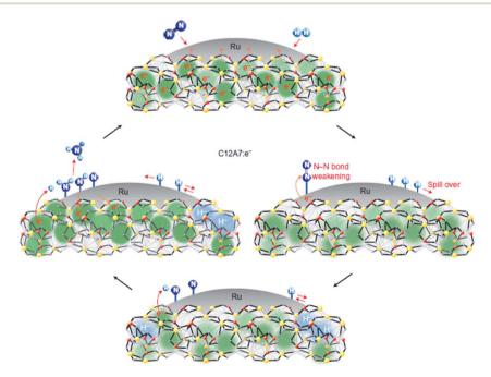
Fig. 23 Possible pathway for the ammonia synthesis reaction over Ru/C12A7:e<sup>-</sup>. Copyright 2012, Springer Nature.
