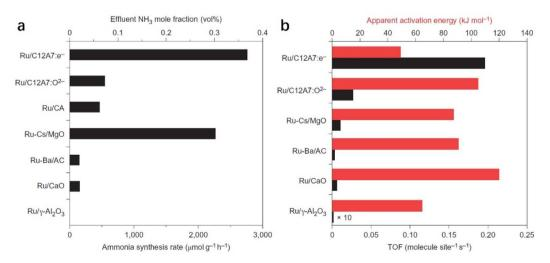
Fig. 4 (a) Catalytic performance for  $NH_3$  synthesis over various Ru (1 wt%)-loaded catalysts at 400 °C and 0.1 MPa. (b) TOFs and apparent activation energies of various Ru (1 wt%)-loaded catalysts for ammonia synthesis. Copyright 2012, Springer Nature.
