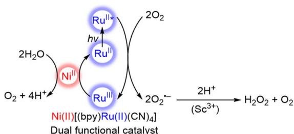
Scheme 2 Catalytic mechanism for the formation of hydrogen peroxide from water and dioxygen with a dual functional catalyst,  $\text{Ni}(\text{II})[(\text{bpy})\text{Ru}(\text{II})(\text{CN})_4]$ , under visible light irradiation.<sup>71</sup>
