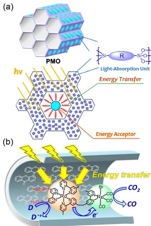
Fig. 7 (a) Structural arrangement of each part of the PMO. (b) Photocatalytic CO<sub>2</sub> reduction by light harvesting hybrids of PRu-Re and 10-Me-acridone in PMO. Reprinted from ref. 121 with permission from American Chemical Society (Copyright 2022).
