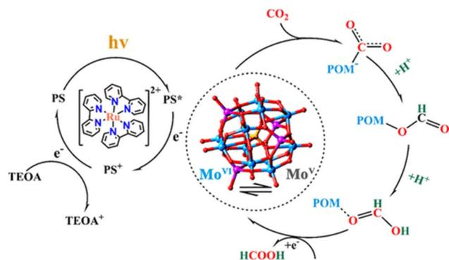
Scheme 7 Proposed mechanism for the photocatalytic  $\text{CO}_2$  reduction to  $\text{HCO}_2\text{H}$  catalyzed by NNU-29. Reprinted from ref. 88 with permission from American Chemical Society (Copyright 2019).
