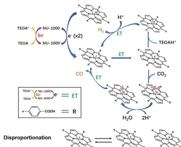
Scheme 9 Proposed mechanism for photocatalytic reduction of  $\text{CO}_2$  using an  $\text{Fe}$ -TCPP@NU-1000 heterogeneous catalyst with TEOA as a sacrificial agent. Reprinted from ref. 90 with permission from Elsevier (Copyright 2022).
