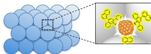
**Fig. 5** Structure of the catalyst prepared with silica–alumina NPs (Al-SiO<sub>2</sub>NPs) supporting QuPh<sup>+</sup>-NA on silica–alumina and PtNPs. Reproduced from ref. 117 with permission from John Wiley and Sons (Copyright 2016).
