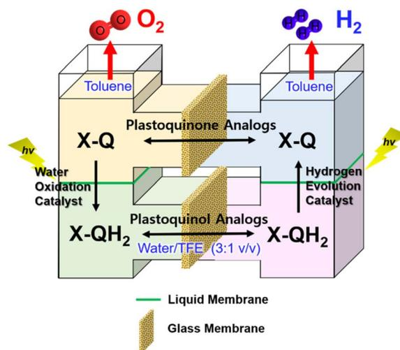
Fig. 8 An O-type photocatalytic cell for photocatalytic H<sub>2</sub>O oxidation and reduction with a combination of PSI and PSII models. Reprinted from ref. 159 with permission from American Chemical Society (Copyright 2022).
