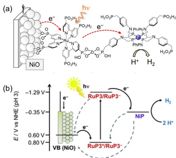
**Scheme 17** (a) Schematic procedure of sequential immersion of  $Zr^{4+}$  bridge-based photocathodes ( $NiO/RuP_3-Zr^{4+}-NiP$ ). (b) Energy diagram of photoinduced electron injection from a  $NiO$  photocathode to the excited state of  $RuP_3$ . Back solid arrows show forward electron transfer and grey dashed arrows show possible recombination pathways between p- $NiO$ ,  $RuP_3$  and  $NiP$ . Reprinted from ref. 134 with permission from the Royal Society of Chemistry (Copyright 2016).
