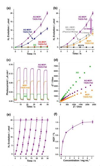
Fig. 6 (a and b) Photocatalytic hydrogen evolution (average values of five sets) by AG, AG-MOP-TADS-Pds, MOP-TADS-Pd2, a mixture of AG and MOP-TADS-Pd2, and AG-Pd (300 W Xe lamp, 10 v/v% TEOA as an electron sacrificer). (c) Photoelectrochemical studies and (d) Nyquist plots of AG-MOP-TADS-Pd2, MOP-TADS-Pd2, and AG. (e) Cycling tests and (f) AQYs (@420 nm) of photocatalytic hydrogen evolution by AG-MOP-TADS-Pd2.
