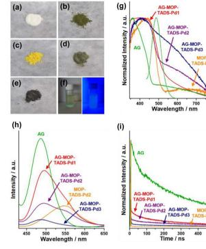
Fig. 5 Photographs of (a) AG, (b) MOP–TADS–Pd2, (c) AG–MOP–TADS–Pd1, (d) AG–MOP–TADS–Pd2, (e) AG–MOP–TADS–Pd3, and (f) an aqueous suspension of AG–MOP–TADS–Pd2 before and after light irradiation. (g) Absorption and (h) emission spectra ( $\lambda_{ex}$  360 nm) and (i) emission decay curves of AG, AG–MOP–TADS–Pds, and MOP–TADS–Pd2. The emission of AG is indicated by a dotted line in (g).
