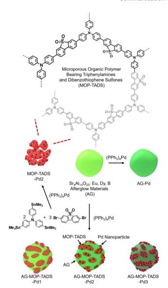
Fig. 2 Synthesis of the composites (AG-MOP-TADS-Pds) of AG, MOP bearing triphenylamines and dibenzothiophene sulfones, and Pd and their control materials (AG-Pd, MOP-TADS-Pd2).
