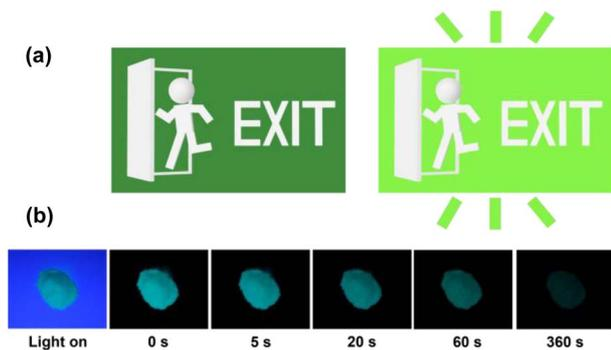
Fig. 1 (a) An example of the application of afterglow phosphorescent materials in common life. (b) Afterglow properties of commercial  $\text{Sr}_4\text{Al}_{14}\text{O}_{25}:\text{Eu},\text{Dy},\text{B}$  used in this study.
