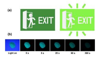
Fig. 1 (a) An example of the application of afterglow phosphorescent materials in common life. (b) Afterglow properties of commercial  $Sr_4Al_{14}O_{25}$ :Eu,Dy,B used in this study.
