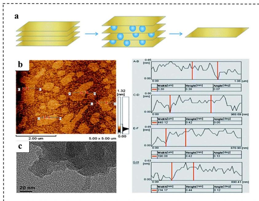
Fig. 7 (a) Illustration of the synthetic strategy of monolayer  $g\text{-C}_3\text{N}_4$  nanosheets. (b) AFM images and (c) TEM images of the as-prepared monolayer  $g\text{-C}_3\text{N}_4$  nanosheets. The right panel shows the height and width information of different nanosheets from the AFM images. Reproduced with permission from ref. 89. Copyright 2013, Royal Society of Chemistry.
