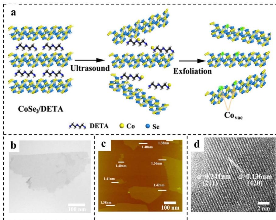
Fig. 6 (a) Schematic of the formation of vacancies in  $\text{CoSe}_2$  ultrathin nanosheets. Characterization of  $\text{CoSe}_2$  ultrathin nanosheets: (b) TEM image; (c) AFM image; (d) HRTEM image. Reproduced with permission from ref. 85. Copyright 2014, American Chemical Society.
