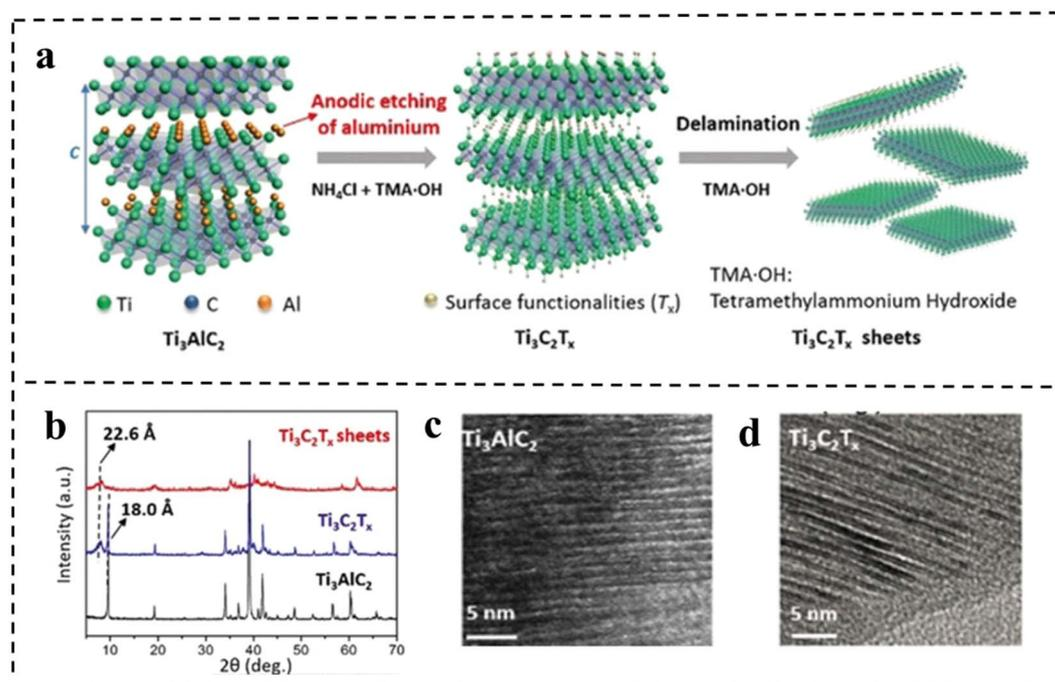
Fig. 11 (a) Schematic of the etching and delamination process of bulk Ti<sub>3</sub>AlC<sub>2</sub>. (b) XRD patterns of Ti<sub>3</sub>AlC<sub>2</sub> and Ti<sub>3</sub>C<sub>2</sub>T<sub>x</sub>. HRTEM images of (c) Ti<sub>3</sub>AlC<sub>2</sub> and (d) Ti<sub>3</sub>C<sub>2</sub>T<sub>x</sub>, respectively. Reproduced with permission from ref. 101. Copyright 2018, Wiley-VCH.
