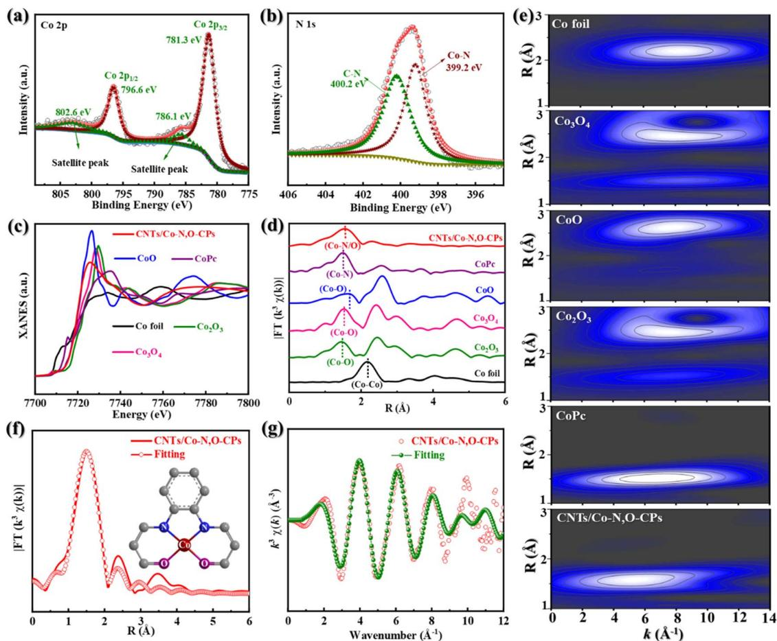
Fig. 2 High-resolution XPS spectra of (a) Co 2p and (b) N 1s of CNTs/Co-N,O-CPs. (c) Co K-edge XANES spectra, (d) FT-EXAFS spectra, and (e) WT-EXAFS images of CNTs/Co-N,O-CPs, Co foil, CoO, Co<sub>3</sub>O<sub>4</sub>, Co<sub>2</sub>O<sub>3</sub> and CoPc. EXAFS fitting curves of CNTs/Co-N,O-CPs in (f) *R* space and (g) *k* space.
