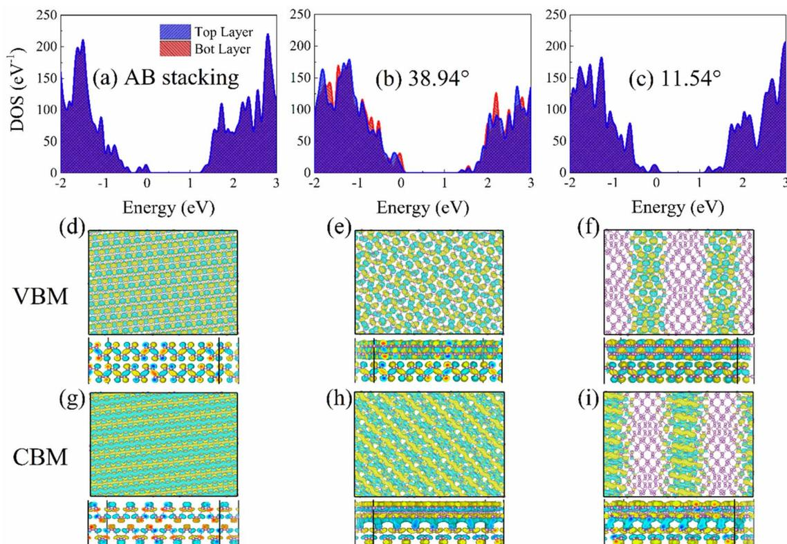
Fig. 4 Electronic structures. Density of states (DOS) of bilayer BP for (a) AB stacking, (b) 39.84°, and (c) 11.54° twist angles, calculated using the CP2K package.<sup>56</sup> The contributions to the DOSs are separated into the top and bottom-layer BP. The Fermi level is set to zero. (d–i) Charge densities of VBM and CBM of bilayer BP. The mismatched potentials separate the electron and hole in the 11.54° system (Fig. S7†), reducing NA coupling.
