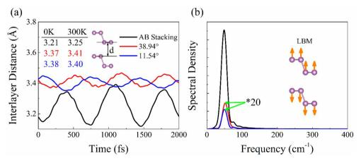
Fig. 3 (a) Evolution of interlayer distance in bilayer BP with AB stacking, 38.94°, and 11.54° twist angles. (b) Spectral density obtained using Fourier transforms of the distance in (a). The peak located at about 50 cm<sup>-1</sup> associated with the low-frequency out-of-plane vibration corresponds to LBM in Raman spectroscopy.<sup>45</sup> The stronger fluctuation of the interlayer distance leads to the higher intensity of the LBM in the AB stacking.
