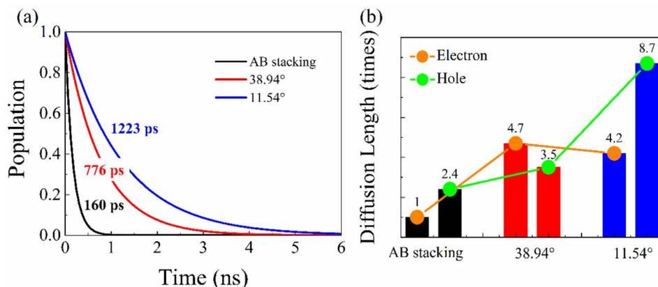
Fig. 6 (a) Nonradiative electron–hole recombination dynamics in AB stacking, and bilayer BP with 38.94° and 11.54° twist angles. (b) The relationship between the charge carrier diffusion length and the stacking configurations. The diffusion lengths increase in the systems with twist angles, which extends the charge carrier lifetimes by decreasing the NACs. The electron diffusion length of AB stacking is set to 1.
