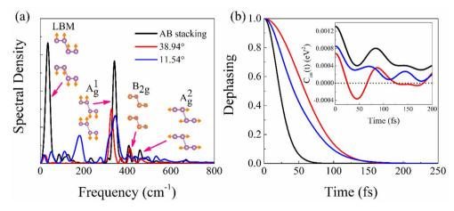
Fig. 5 (a) Spectral densities obtained using Fourier transforms of the un-ACF of the bandgap fluctuations and (b) pure-dephasing functions. The inset of (b) shows the un-ACF,  $C_{\rm un}(t)$ , whose starting value equals the bandgap squared. The larger initial value generally leads to faster pure-dephasing.
