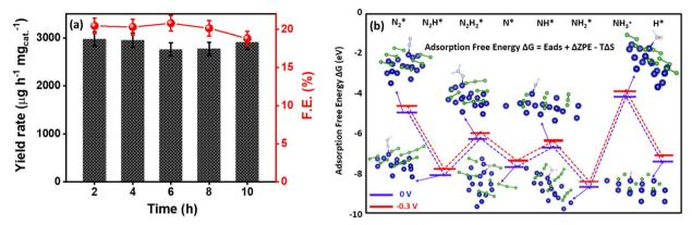
Fig. 4 (a) F.E. and NH<sub>3</sub> yield obtained after chronoamperometry tests performed for 10 h under N<sub>2</sub>-saturated 0.1 M KOH for Co<sub>2</sub>B (1:8). (b) Free energy diagrams of the NRR distal pathway on  $Co_2B$  surface (Co active site) at applied potentials of 0 and -0.3 V and H<sup>+</sup> adsorption at identical potentials
