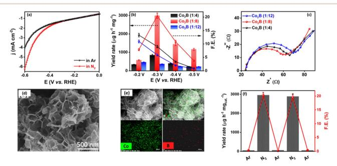
Fig. 1 (a) Linear sweep voltammograms for Co<sub>2</sub>B (1:8) in Ar- and N<sub>2</sub>-saturated 0.1 M KOH, (b) comparison of yield rates and F.E. of Co<sub>2</sub>B catalysts at different applied potentials, (c) Nyquist plots, (d) FE-SEM image of Co<sub>2</sub>B (1:8) and (e) corresponding elemental dot mapping showing uniform distribution of Co and B elements over the scanned area. (f) F.E. and yield rates obtained during NRR under switching gas-feed (Ar/N<sub>2</sub>) environments.
