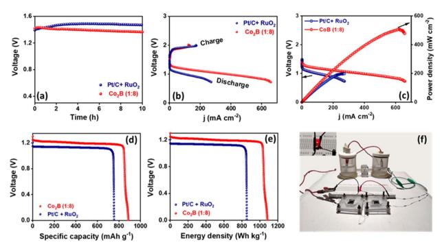
Fig. 6 (a) Open circuit voltage, (b) charge—discharge polarization curves, (c) power density plots extracted from discharge polarization curve for Zn-air battery assembled using  $Co_2B$  (1:8) and Pt/C as an air cathode. (d) Corresponding specific capacity and (e) energy density curves obtained at 10 mA cm<sup>-2</sup>. (f) Photograph of Zn-air battery-powered NRR full cell setup (air cathode in battery:  $Co_2B$  (1:8); cathode and anode in NRR full cell:  $Co_2B$  (1:8)).
