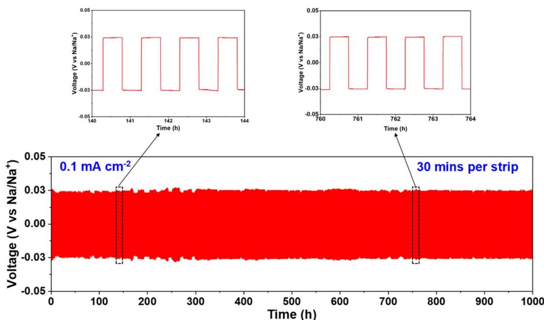
Fig. 4 Long-term stability of galvanostatic cycling at 0.1 mA cm<sup>-2</sup> at 25 °C for 1000 h using Na|NGS15|Na symmetric cell.
