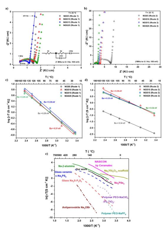
Fig. 3 (a) and (b) RT-impedance for NGS5–20 prepared *via* routes 1 and 2, respectively. (c) and (d) Arrhenius plots for NGS5–20 prepared *via* routes 1 and 2, respectively, and (e) Arrhenius plot of solid electrolytes compared with NGS15.<sup>38,41,44</sup>
