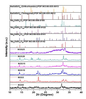
Fig. 1 PXRD patterns of NGS0-NGS25 prepared by route 1 along with the reference patterns of Na $_3$ GdSi $_3$ O $_9$  (PDF: 00-035-0142), Na $_5$ GdSi $_4$ O $_{12}$  (PDF: 00-035-0141) (rhombohedral), Na $_9$ GdSi $_6$ O $_{18}$  (PDF 00-056-0122), Na $_3$ GdSi $_2$ O $_7$  (PDF: 00-056-0185) (hexagonal), NaGdSiO $_4$  (orthorhombic phase; PDF: 00-035-0013), and NaGdSiO $_4$  (tetragonal phase; PDF: 00-035-0012).
