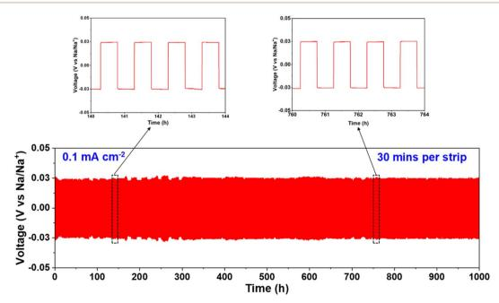
Fig. 4 Long-term stability of galvanostatic cycling at 0.1 mA cm<sup>-2</sup> at 25 °C for 1000 h using Na|NGS15|Na symmetric cell.
