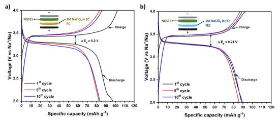
Fig. 5 Galvanostatic charge-discharge curves at 0.1C at 25 °C. (a) Na|NGS15|20 μL of 1 M NaClO<sub>4</sub> in EC:PC|NVP and (b) Na|NGS15|20 μL of 1 M NaClO<sub>4</sub> in PC:FEC|NVP (NGS15 was prepared via route 1).
