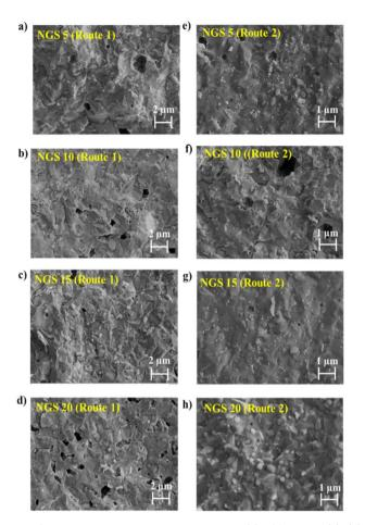
Fig. 2 SEM images of the cross-section of NGS5-20 pellets (a)-(d) route 1 and (e)-(h) route 2, respectively.
