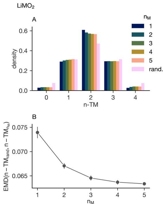
Fig. 3 (A) Histogram showing the occurrence of the different possible  $n$ -TM sites in Monte Carlo simulated  $\text{LiMO}_2$ , where M is all equimolar charge-balanced combinations of Mn(III), Cr(III), Fe(III), Ni(II) and Ti(IV). (B) The Earth Mover's Distance (EMD) between the Monte Carlo sampled distributions of  $n$ -TM sites, and the fully random distribution. The error bars show the 95% confidence interval in the EMD.
