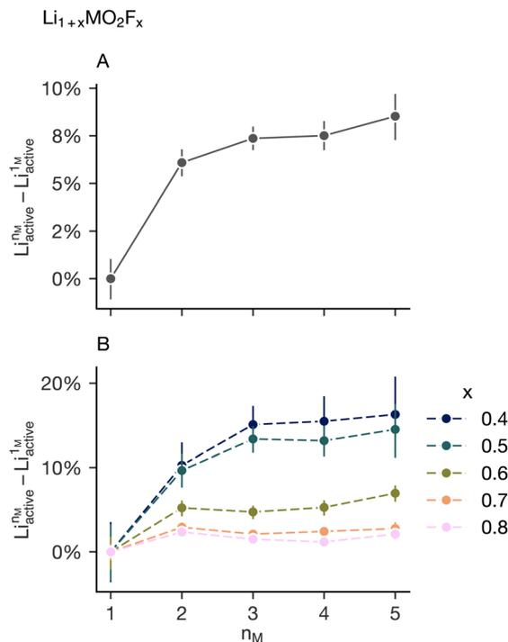
Fig. 4 (A) The mean change in active lithium in a  $\text{Li}_{1+x}\text{MO}_2\text{F}_x$  as a function of the number of transition metals in the Monte Carlo simulation, relative to the average percolating lithium in single transition metal systems decomposed by the lithium excess and fluorine content. The error bars show the 95% confidence interval in the active lithium fraction. (B) Showing the same data, but decomposed per value of  $x$ .
