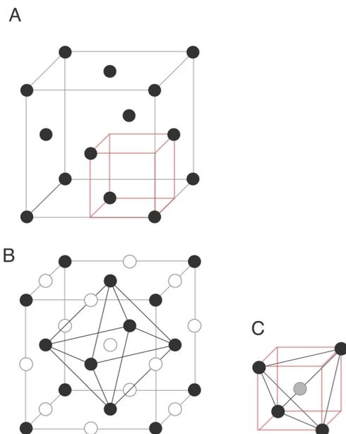
**Fig. 1** (A) Face-centered cubic (FCC) lattice, such as the one exhibited by  $\text{O}^{2-}$  ions in many lithium-transition metal oxides. (B) Octahedral holes in the FCC lattice (white) that may be filled by cations in a lithium-transition metal oxide. (C) Tetrahedral holes (grey) which form the transition states for lithium diffusion in a disordered rock salt cathode material.
