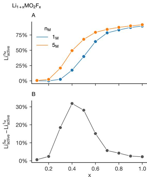
Fig. 5 (A) The change in the mean active lithium percentage as a function of  $x$  in  $\text{Li}_{1+x}\text{MnO}_2\text{F}_x$  and  $\text{Li}_{1+x}\text{Mn}_{0.2}\text{Cr}_{0.2}\text{Fe}_{0.2}\text{Ni}_{0.2}\text{Ti}_{0.2}\text{O}_2\text{F}_x$  as a function of  $x$ . (B) The difference between the two trends shown in plot (A).
