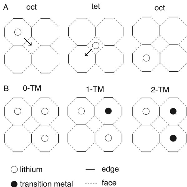
**Fig. 2** (A) 2D representation of the oct–tet–oct hop of a lithium ion diffusing in a rock salt structured cathode material. (B) 2D representation of the different face sharing ions for the transition-state tetrahedral site in the oct–tet–oct hop. The energy barrier for the hop will increase as a function of the number of transition metals face-sharing with the tetrahedral site.
