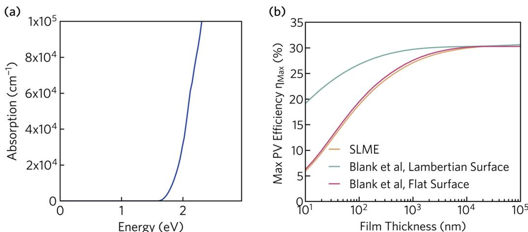
**Fig. 5** (a) Optical absorption spectrum of  $\text{K}_2\text{CsSb}$  calculated using HSE + SOC. (b) Thickness-dependent theoretical maximum efficiency of  $\text{K}_2\text{CsSb}$  calculated using the “spectroscopic limited maximum efficiency” (SLME) method and detailed balance metric proposed by Blank *et al.*<sup>40</sup>
