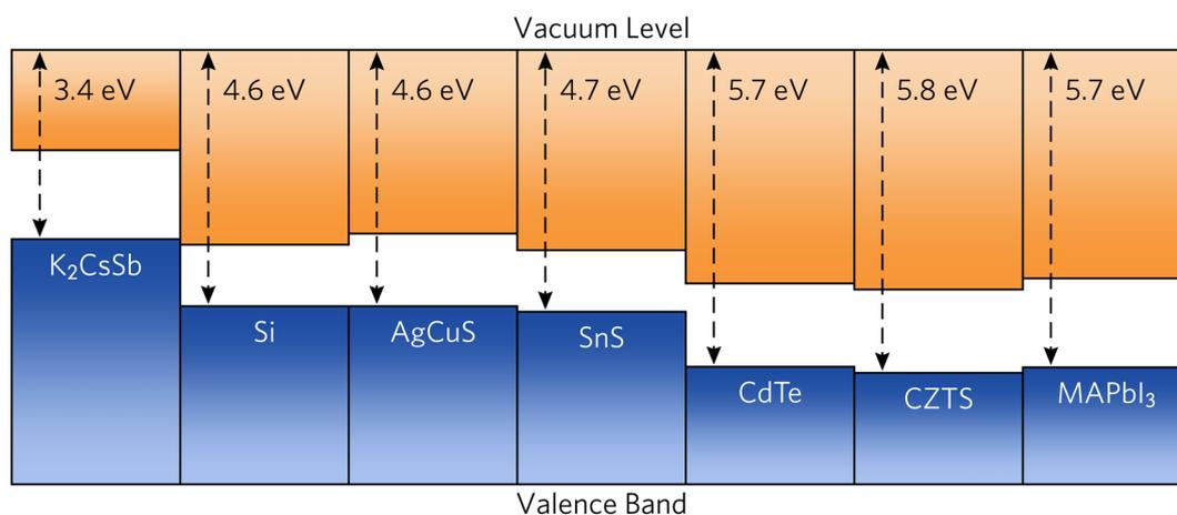
Fig. 6 Calculated band alignment of  $\text{K}_2\text{CsSb}$  compared to conventional and emerging photovoltaic absorbers. Electron affinity and bandgap data were taken from ref. 63–66.
