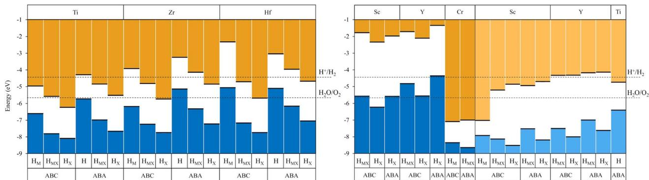
Fig. 10 VBM and CBM alignments with respect to  $\text{H}^+/\text{H}_2$  and  $\text{H}_2\text{O}/\text{O}_2$  potential energy levels for group IV C-MXenes (left) and group III,  $\text{Cr}_2\text{CO}_2$ , and  $\text{Ti}_2\text{NO}_2$  MXenes (right). The blue and orange bars indicate the VB and CB, respectively, and darker and lighter colours represent C- and N-MXenes, respectively.
