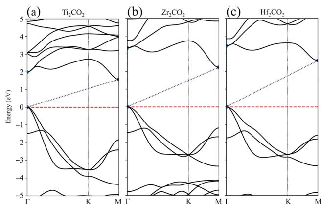
Fig. 8 PBE0 band structure for (a)  $\text{Ti}_2\text{CO}_2$ , (b)  $\text{Zr}_2\text{CO}_2$ , and (c)  $\text{Hf}_2\text{CO}_2$  in their most stable structure, ABC  $\text{H}_M$ . The blue-dotted line indicates the bandgap from the VBM to the CBM. The red-dashed line indicates the Fermi level,  $E_F$ , made to coincide with the VBM, to which all energies have been referenced.
