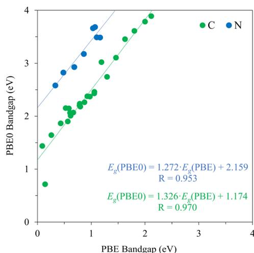
Fig. 13 Linear correlations between PBE0 and PBE  $E_g$  values, alongside the linear equation  $E_g(\text{PBE0}) = a \times E_g(\text{PBE}) + b$ , and the regression coefficient,  $R$ . Green and blue dots denote C-MXene and N-MXene values, respectively.
