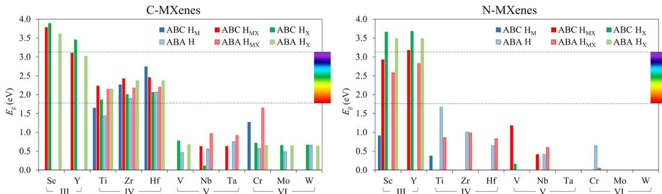
Fig. 7 Calculated bandgap,  $E_g$ , in eV, with the PBE0 functional, for the studied O-terminated MXenes in the six different O-terminated configurations. On the left (right) are represented the C-MXenes (N-MXenes). In each plot the range of the visible spectrum is displayed, from 1.8 to 3.1 eV.
