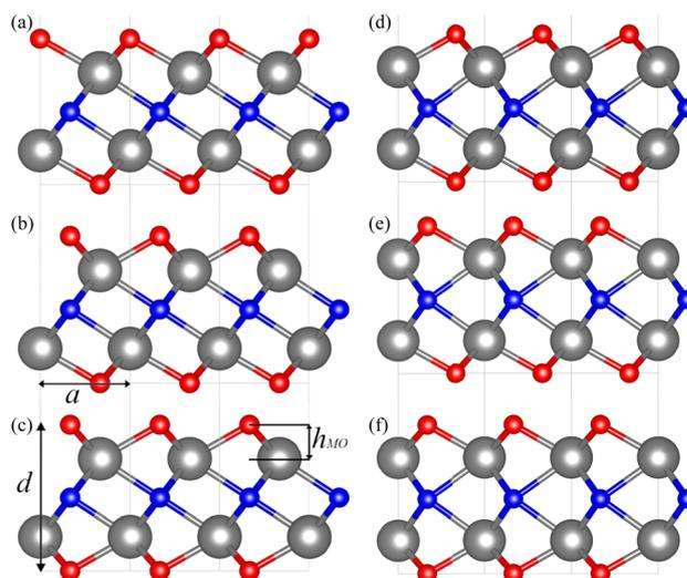
Fig. 2 Side views of the six possible configurations for an O-terminated MXene. (a)–(c) represent the  $H_M$ ,  $H_{MX}$ , and  $H_X$  configurations for the ABC stacking, while (d)–(f) represent the H,  $H_{MX}$ , and  $H_X$  structures for ABA stacking, respectively. O atoms are shown as red spheres. The rest of the colour coding is as in Fig. 1. The lattice parameter,  $a$ , width,  $d$ , and M–O interplanar distance,  $h_{MO}$ , are represented by black arrows.
