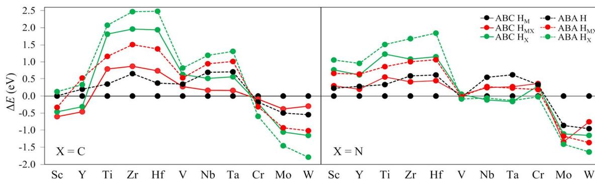
Fig. 5 Relative energy differences,  $\Delta E$ , in eV, for each O-functionalized MXene, with respect to the ABC  $H_M$  case, considering ABC/ABA stacking and different hollow positions. The left (right) panel represents the C-MXenes (N-MXenes).
