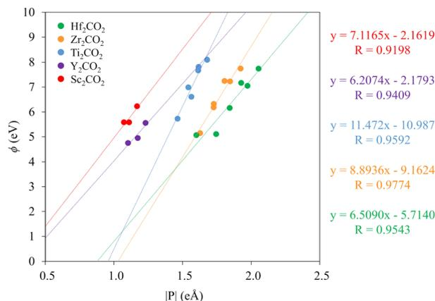
Fig. 12 Relation between the work function,  $\phi$ , and the absolute surface dipole moment,  $P$ , for the group III and IV C-MXenes. On the right are present the colour coded linear regression equations.
