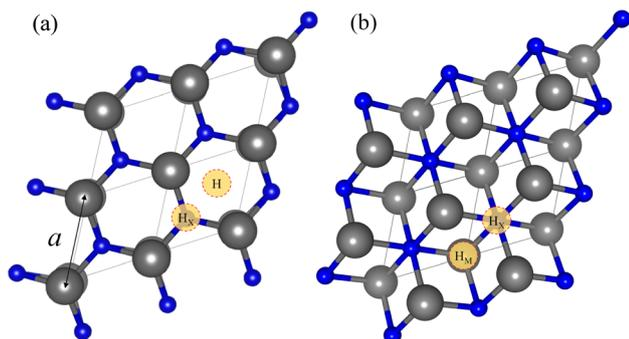
Fig. 1 Top view of the pristine MXene structures with (a) ABA and (b) ABC stacking. The yellow circles mark high symmetry sites where a termination could be placed –H stands for hollow,  $H_M$  for metal hollow and  $H_X$  for carbon/nitrogen hollow. The transition metal (M) and C or N (X) are represented by grey and blue spheres, respectively. The  $p(1 \times 1)$  unit cell is indicated by grey lines, and the cell parameter,  $a$ , by a black arrow.
