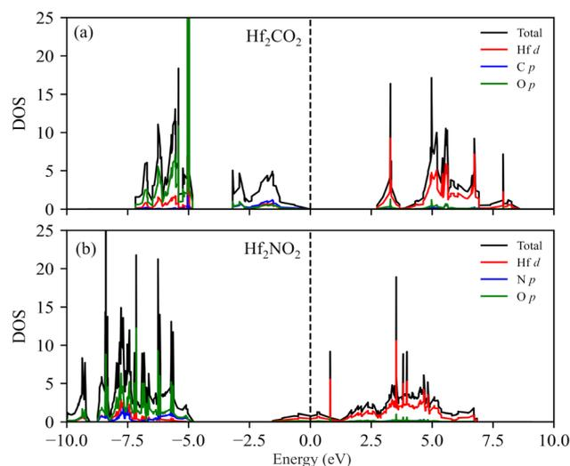
Fig. 6 Total and projected DOS calculated at the PBE0 level for (a)  $Hf_2CO_2$  and (b)  $Hf_2NO_2$  in their most stable structure, ABC stacking and oxygens in  $H_M$ , referenced to the VBM and  $E_F$  levels, respectively.
