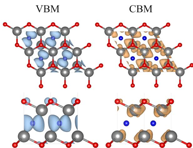
Fig. 11 Charge density of the VBM (left, indicated with a blue surface) and CBM (right, indicated with an orange surface) of the  $\text{Zr}_2\text{CO}_2$  MXene with ABC stacking and  $\text{H}_\text{M}$  structure, computed at the PBE0 level. Both surfaces have an isovalue of  $0.015 \text{ e} \text{ \AA}^{-3}$ . The upper images represent the top views, while the lower ones represent the side views of the MXene.
