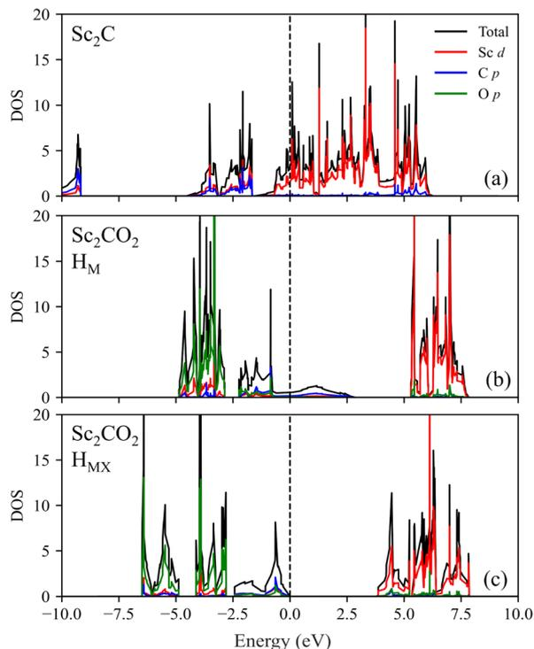
Fig. 9 Total and projected DOS comparison of (a)  $\text{Sc}_2\text{C}$  (PBE) and  $\text{Sc}_2\text{CO}_2$  (PBE0) with (b)  $\text{H}_\text{M}$  or (c)  $\text{H}_\text{MX}$  structures, all with ABC stacking. The energy levels are displayed with respect to the  $E_\text{F}$  level except for  $\text{Sc}_2\text{CO}_2$   $\text{H}_\text{MX}$ , referenced to the VBM.
