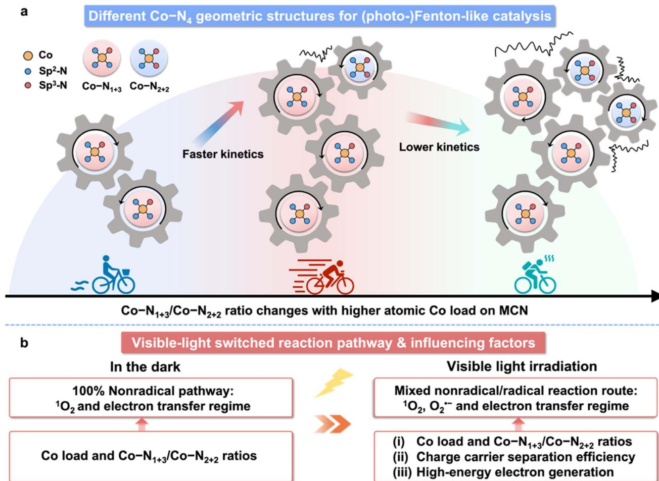
Scheme 2 (a) Schematic illustration of different Co-N<sub>4</sub> geometric configurations for (photo-)Fenton-like catalysis. (b) Visible-light switched reaction pathway and factors related to catalysis in (photo-)Fenton-like reactions with Co-MCN SACs.
