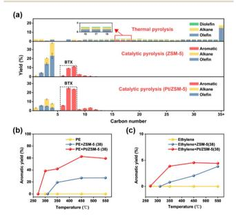
Fig. 4 (a) Product distribution from thermal pyrolysis (500 °C) and catalytic pyrolysis (450 °C) of PE. (b) Total yield of aromatics from thermal/catalytic pyrolysis of PE at different temperatures. (c) Total yield of aromatics from catalytic conversion of ethylene at different temperatures.
