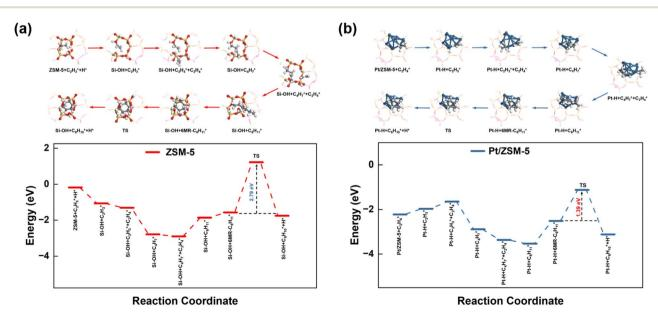
Fig. 5 Reaction energy diagram of ethylene oligomerization, cyclization and dehydrogenation to the benzene precursor over (a) ZSM-5 (38) and (b) Pt/ZSM-5 (38). (Pink: Al, yellow: Si, red: O, grey: C, white: H, and blue: Pt.)
