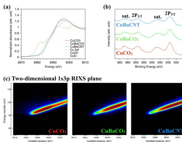
Fig. 2 (a) X-ray absorption near-edge structures and (b) X-ray photoelectron spectroscopy of  $\text{CuCO}_3$ ,  $\text{CuBaCO}_3$ , and CuBaCNT. (c) Two-dimensional 1s3p RIXS plane of  $\text{CuCO}_3$ ,  $\text{CuBaCO}_3$ , and CuBaCNT (energy transfer from 3d to 3p of Cu orbitals).
