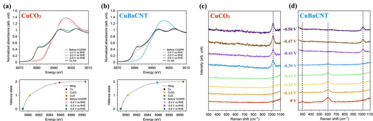
Fig. 4 Operando X-ray absorption near-edge structure and valence-state analyses of (a) CuCO<sub>3</sub> and (b) CuBaCNT during the CO<sub>2</sub>RR in a flow cell. Operando Raman spectroscopy of (c) CuCO<sub>3</sub> and (d) CuBaCNT. The voltage is vs. RHE.
