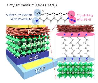
Fig. 1 Schematic illustration of perovskite solar cells with cross-linkable molecule, octylammonium azide ( $OAN_3$ ).
