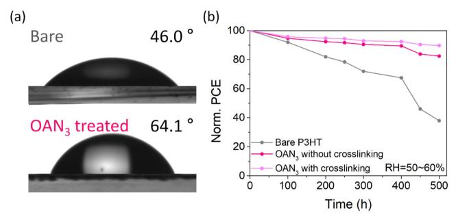
Fig. 5 (a) Contact angles of perovskite film before and after OAN<sub>3</sub> treatment. (b) Moisture-stability under RH: 50-60% storage for PSCs with bare, OAN3 treated non-crosslinking, and after crosslinking.
