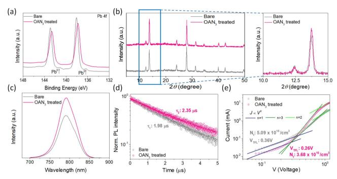
Fig. 3 (a) XPS spectrum of Pb 4f before and after OAN3 introduction. (b) XRD spectrum of perovskite film under various conditions. (c) Steadystate and (d) time-resolved photoluminescence schematic illustration of perovskite solar cells with and without OAN3. (e) Space charge limited current measurement for hole-only devices with and without OAN<sub>3</sub>.
