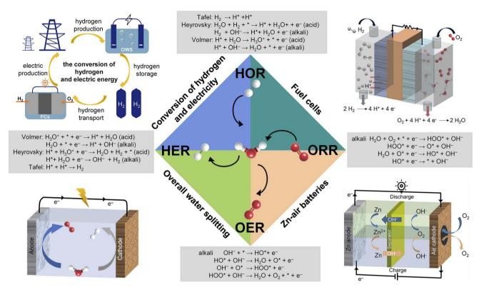
Fig. 1 A green cycle between hydrogen and electricity, hydrogen electrocatalyst reaction type and mechanism under acidic/alkaline conditions (\* represents the catalytic active site), oxygen electrocatalyst reaction type and mechanism under alkaline conditions, and schematic illustrations of OWS, ZABs, and FCs.
