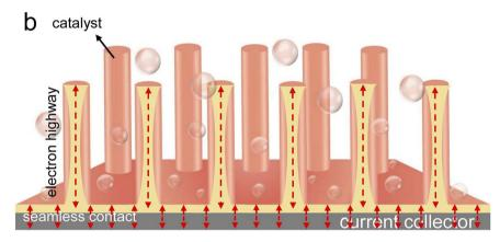
Fig. 2 Schematic of the internal structure of (a) powdery electrode, in which electrocatalysts are coated on the current collector with the aid of a polymer binder and conductive additives, and (b) self-supporting electrode, in which electrocatalysts are grown directly on the current collector.
