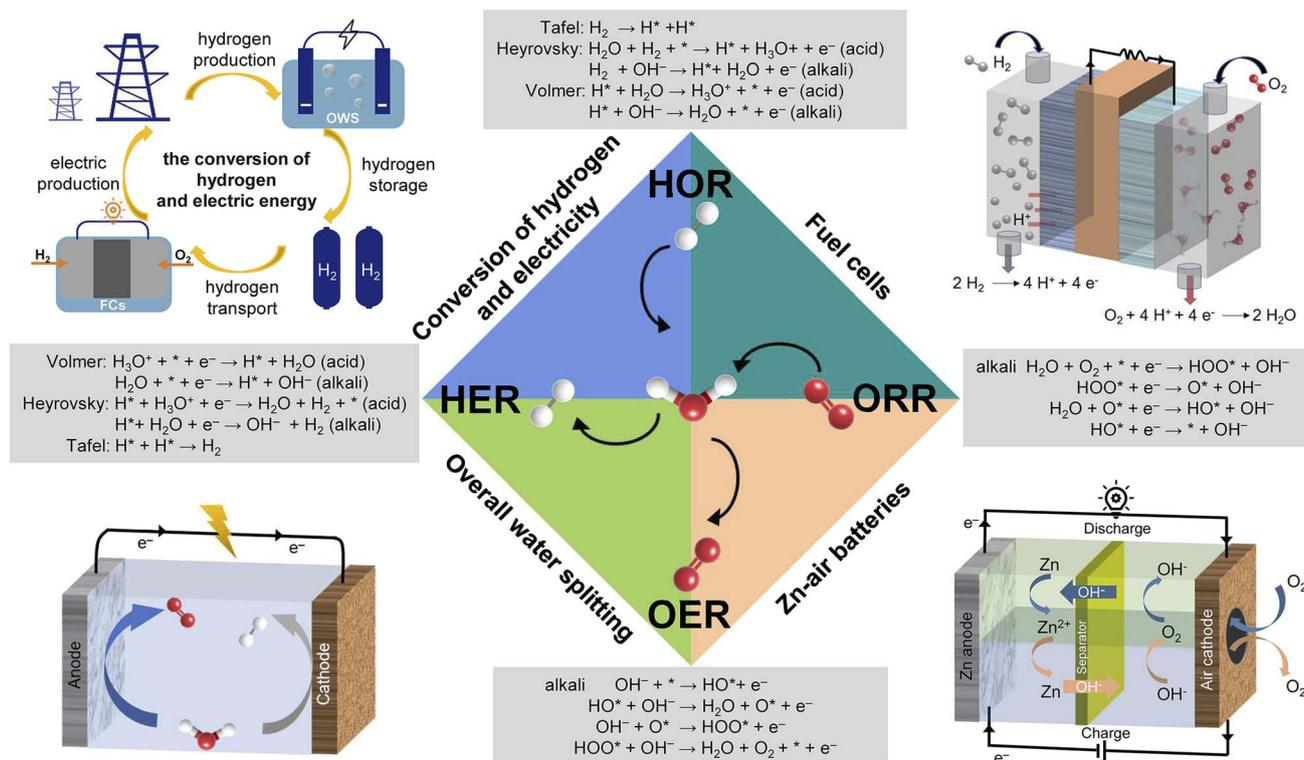
Fig. 1 A green cycle between hydrogen and electricity, hydrogen electrocatalyst reaction type and mechanism under acidic/alkaline conditions (\* represents the catalytic active site), oxygen electrocatalyst reaction type and mechanism under alkaline conditions, and schematic illustrations of OWS, ZABs, and FCs.
