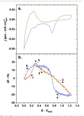
Fig. 4 Mass changes due to hydrogen adsorption, absorption, and desorption behaviors induce frequency changes on pure Pd crystals during conditioning as shown by (a) CV and (b) E-QCM measurements with anodic scans in orange and cathodic scans in blue. Reaction conditions: 5 mV s<sup>-1</sup> scan rate, Ar-saturated 0.1 M KOH solution.
