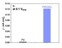
Fig. 2 The presence of  $CeO_2$  has a significant impact on hydrogen and oxygen interactions with Pd and leads to better HOR performance as shown in (a) CV at a 50 mV s<sup>-1</sup> scan rate in Ar-saturated 0.1 M KOH, (b) HOR performed in H<sub>2</sub>-saturated 0.1 M KOH at 5 mV s<sup>-1</sup> and 1600 rpm and (c) comparison of specific activity at 0.1  $V_{RHE}$  on pure Pd (black) and Pd/CeO<sub>2</sub> (blue).
