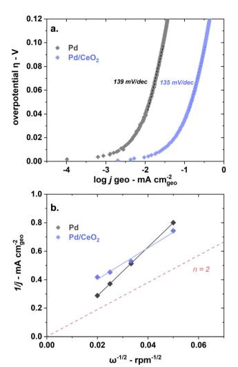
Fig. 3 Pd and Pd/CeO<sub>2</sub> show similar Tafel slopes but different estimated number of transferred electrons as shown in (a) a Tafel plot obtained at 5 mV s<sup>-1</sup> and 1600 rpm and (b) Koutecky-Levich plot obtained at 0.8  $V_{\rm RHE}$  with measurements at 400, 900, 1600 and 2500 rpm at 50 mV s<sup>-1</sup>. Both reactions were performed in  $H_2$ -saturated 0.1 M KOH.
