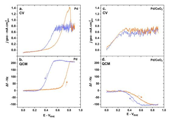
Fig. 6 E-QCM reveals fundamental differences during HOR on Pd and Pd/CeO<sub>2</sub> as shown by (a) the measured current density during CV and (b) simultaneous E-QCM measurements on pure Pd; (c) measured current density during CV and (d) simultaneous E-QCM measurements on Pd/CeO<sub>2</sub>. The anodic scans are represented in orange and the cathodic scans in blue. Reaction conditions: 5 mV s<sup>-1</sup> scan rate, H<sub>2</sub>-saturated 0.1 M KOH solution.
