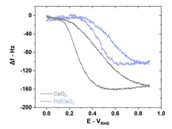
Fig. 7 EQCM measurements on pure  $CeO_2$  reveals the role played by the support on  $Pd/CeO_2$  represented by the difference in frequency during HOR. Reaction conditions: 5 mV s<sup>-1</sup> scan rate, H<sub>2</sub>-saturated 0.1 M KOH solution.
