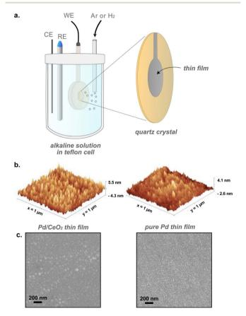
Fig. 1 (a) Schematic showing the setup used for *in situ* electrochemical characterization of thin films using E-QCM. RE, CE and WE refer to reference, counter and working electrodes, respectively. (b) Atomic force microscopy and (c) scanning electron microscopy images of  $Pd/CeO_2$  and pure Pd thin films prepared by evaporation.
