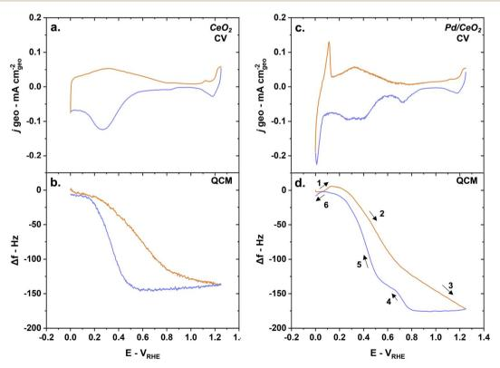
Fig. 5 The mass changes measured on  $Pd/CeO_2$  are dominated by adsorption and desorption phenomena occurring on  $CeO_2$  during conditioning as shown by (a) CV on  $CeO_2$  and simultaneous (b) QCM measurements and (c) CV on  $Pd/CeO_2$  and simultaneous (d) QCM measurements. The anodic scans are represented in orange while the cathodic scans are in blue. Reaction conditions: 5 mV s<sup>-1</sup> scan rate, Arsaturated 0.1 M KOH solution.
