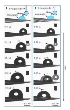
Fig. 2 Optical microscopic observation of the main droplet to determine the critical droplet motion volume on the straight (a) and helical (b) micro-grooved cones. With continuous feeding of water, the main droplet moves from the tip to the base of the cone. The critical droplet motion volume on the helical micro-grooved cone is smaller than that on the straight micro-grooved cone.
