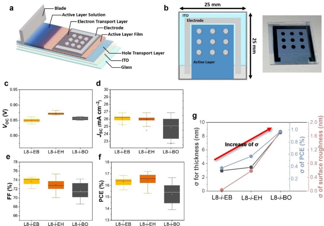
Fig. 5 (a) The schematic illustration of device fabrication *via* the blade-coating process with device configuration. (b) The illustration and picture of the 2.5 cm × 2.5 cm device. Distribution of (c)  $V_{OC}$ , (d)  $J_{SC}$ , (e) FF, and (f) PCE for L8-*i*-EB, L8-*i*-EH, and L8-*i*-BO based 9 devices on 2.5 cm × 2.5 cm substrate. (g) The values of standard deviation for thickness, surface roughness of active layers, and PCEs based on PM6:L8-*i*-EB, PM6:L8-*i*-EH, and PM6:L8-*i*-BO.
