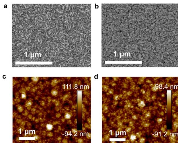
Fig. 1 Top-view SEM and AFM images of  $\text{In}_2\text{S}_3$  buffer layers (a and c) without  $\text{InCl}_3$  post-treatment and (b and d) with post-treatment by using  $0.02\text{ g mL}^{-1}$   $\text{InCl}_3$ .
