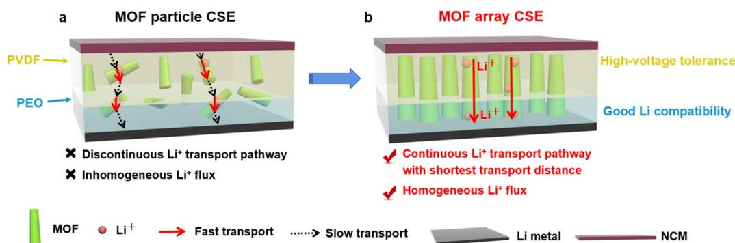
Fig. 2 Schematic illustrations of the Li<sup>+</sup> transport behaviors in (a) the MOF particle CSE and (b) MOF array CSE. The discrete MOF particles in the MOF particle CSE result in a discontinuous Li<sup>+</sup> transport pathway with an inhomogeneous Li<sup>+</sup> flux. Meanwhile, the MOF array CSE not only offers a continuous Li<sup>+</sup> transport pathway with the shortest transport distance between the cathode and anode, but also contributes to the homogeneous Li<sup>+</sup> flux.
