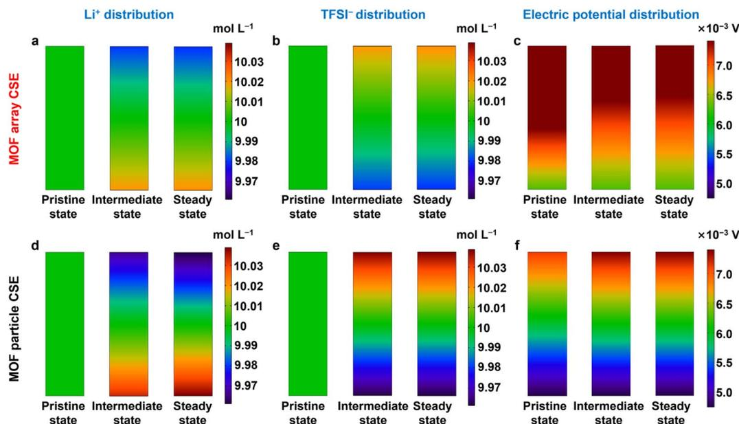
Fig. 5 COMSOL simulation results. The Li<sup>+</sup>, TFSI<sup>-</sup>, and electric potential distribution in (a–c) the MOF array CSE and (d–f) MOF particle CSE at pristine, intermediate, and steady states during Li<sup>+</sup> deposition at a current density of 0.2 mA cm<sup>-2</sup>.
