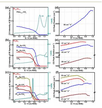
Fig. 4 Integrated peak intensities and peak positions of the various CO species in the COR process plotted against electrode potential change. (a) and (d)  $Pt_{1.8}Au_{0.2}$ , (b) and (e)  $Pt_{1.4}Au_{1.8}$ , (c) and (f)  $Pt_{0.2}Au_{1.8}$ .  $Pt_{rich}Au - CO_L$  (dark yellow line),  $Pt_{adj}Au - CO_L$  (red line),  $Pt_{iso}Au - CO_L$  (blue line),  $CO_B$  (wine-colored line). The cyan solid lines are the COR curves of the PtAu samples in (a), (c) and (e).
