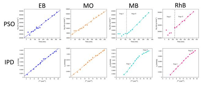
Fig. 6 (Top) Pseudo-second order and (bottom) intra-particle diffusion kinetic models for adsorption of dyes on to LDH/BNOx nanocomposite membranes.
