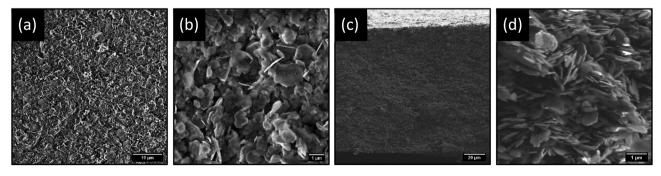
Fig. 2 (a and b) Top-view and (c and d) cross-sectional SEM images of LDH/BNOx membranes. Lower magnification images (a and c) show general uniformity of membranes, and higher magnification (b and d) shows finer membrane structure consisting of networks of nanosheets.
