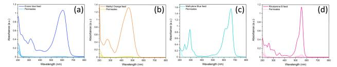
Fig. 5 UV-vis spectra demonstrating the retention of 20 mL of (a) 15  $\mu$ M Evans blue, (b) 50  $\mu$ M methyl orange, (c) 27  $\mu$ M methylene blue, and (d) 20  $\mu$ M rhodamine B by LDH/BNOx nanocomposite membranes.
