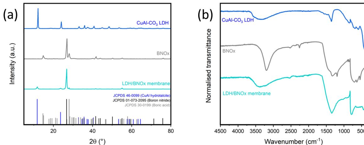
Fig. 1 (a) pXRD patterns and (b) FT-IR spectra of CuAl-CO<sub>3</sub> LDHs (blue), BNOx (grey) and LDH/BNOx nanocomposite (turquoise). pXRD reference patterns are provided for CuAl hydroxalcite, boron nitride and boric acid.
