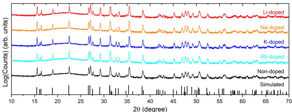
Fig. 2 XRD patterns for CBGTSe films with different dopants, plotted on a log scale to accentuate any possible impurities. The simulated XRD stick pattern for CBGTSe ( $x = 0.7$ ) was simulated using CrystalDiffract software with lattice parameters adapted from Wessler *et al.*<sup>48</sup> XRD patterns of the doped CBGTSe films exhibit only the simulated peaks of the main phase, which excludes significant formation of secondary phases.
