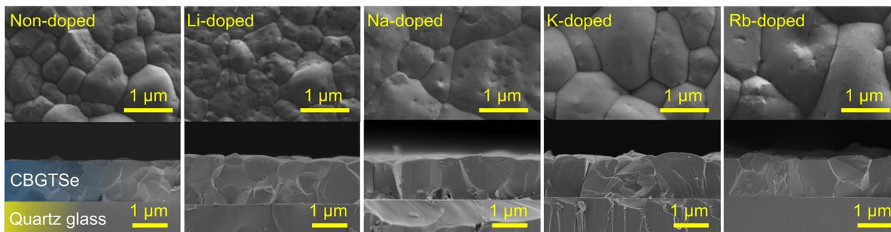
**Fig. 1** Surface/cross-section SEM images of non-doped and alkali (*i.e.*, Li, Na, K, and Rb) doped CBGTSe films deposited on quartz glass substrates. All scale bars represent 1  $\mu\text{m}$ . Note that the alkali-doping was achieved by pre-depositing approximately 4-nm-thick layers of alkali fluoride (*e.g.*, KF). Cross-section images were acquired after depositing  $\sim 5$  nm of Au to avoid surface charging.
