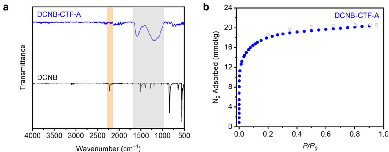
Fig. 6 Solid-state characterization of DCNB-CTF-A made with 5.00 equiv. of  $\text{ZnBr}_2$  at  $400\text{ }^\circ\text{C}$  for 40 h. (a) ATR-IR spectra of DCNB and DCNB-CTF-A. The orange highlighted region shows the disappearance of the  $\text{C}\equiv\text{N}$  stretch from DCNB, and the gray highlighted region indicates the appearance of triazine stretches in DCNB-CTF-A. (b)  $77\text{ K N}_2$  adsorption (filled circles) and desorption (open circles) isotherms of DCNB-CTF-A.
