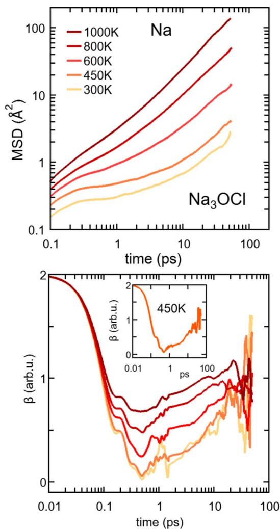
Fig. 11 (Color online) Top: log–log plot of MSD *vs.* time for Na in  $\text{Na}_3\text{OCl}$  at temperatures in between  $T = 300$  K and 1200 K. Bottom: corresponding values of  $\beta$ . Inset:  $\beta$  value as a function of time at  $T = 800$  K. Note that the log–log plots of MSD *vs.* time data for the  $\text{Na}_{3-x}\text{OH}_x\text{Cl}$  ( $x = 0$ ,  $x = 0.5$ , and  $x = 1$ ) systems are reported in the ESI (Fig. S2†).
