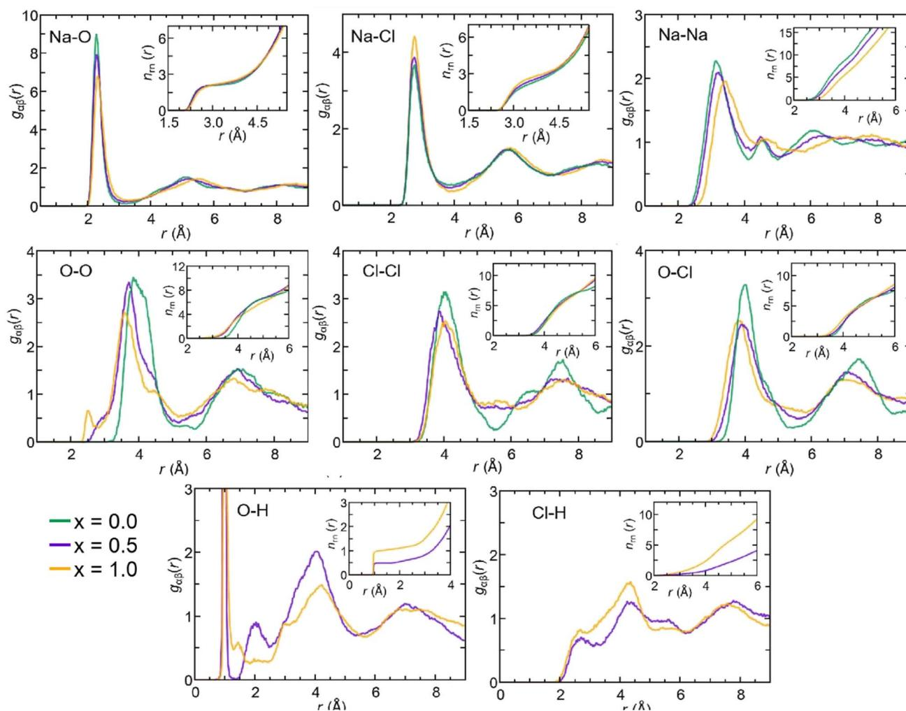
Fig. 4 (Color online) Partial pair correlation functions  $g_{\alpha\beta}(r)$  for amorphous  $\text{Na}_{3-x}\text{OH}_x\text{Cl}$  ( $x = 0$ ,  $x = 0.5$ , and  $x = 1$ ) at  $T = 300$  K relative to the pairs Na–O, Na–Cl, Na–Na, O–O, Cl–Cl, O–Cl, O–H, and Cl–H. The running integrals over the interatomic distance are shown.
