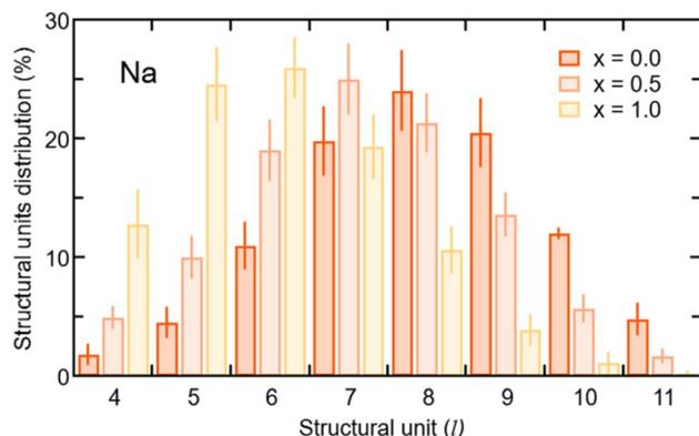
Fig. 6 Distributions of the structural units for Na of amorphous Na<sub>3-x</sub>OH<sub>x</sub>Cl (x = 0, x = 0.5, and x = 1) as a function of the number of neighbors in each unit ( $l$ ). Values obtained by using the definition of "total" coordination  $n_{ij}^t$ , given in Section 3.1.3.
