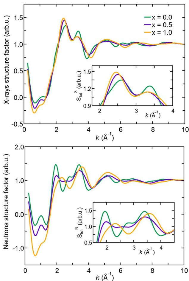
Fig. 2 (Color online) Total X-ray (top) and neutron (bottom) structure factors for amorphous  $\text{Na}_{3-x}\text{OH}_x\text{Cl}$  ( $x = 0$ ,  $x = 0.5$ , and  $x = 1$ ) obtained through Fourier transform of the total pair correlation functions at  $T = 300 \text{ K}$ . Insets: zoomed-in view of the  $1.8\text{--}4.0 \text{ \AA}^{-1}$  and  $1.5\text{--}4.5 \text{ \AA}^{-1}$  ranges, respectively.
