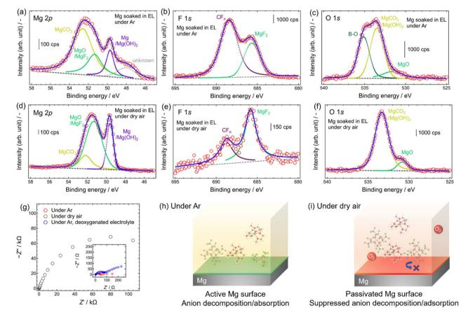
Fig. 2 Surface Mg 2p, F 1s, and O 1s spectra of Mg strips soaked in electrolyte solutions under (a-c) Ar and (d-f) dry-air atmospheres. (g) EIS spectra of symmetric [Mg||Mg] cells. Schematic illustrations of the surface chemistry of magnesium electrodes under (h) Ar and (i) dry-air atmosphere.
