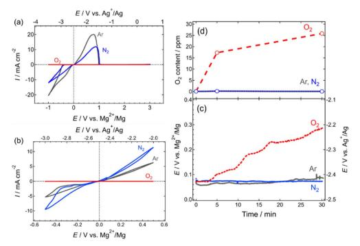
Fig. 1 CV and OCP profiles of Pt and Mg electrodes under steady flow of different gases recorded in 0.3 mol dm $^{-3}$  Mg[B(HFIP)<sub>4</sub>]<sub>2</sub>/G2 electrolytes. CV profiles using (a) Pt and (b) Mg working electrodes. Time profiles of (c) OCV of Mg electrodes and (d) corresponding O<sub>2</sub> concentration in electrolyte solutions. The time profiles of O<sub>2</sub> concentrations under N<sub>2</sub> and Ar were zero during measurements.
