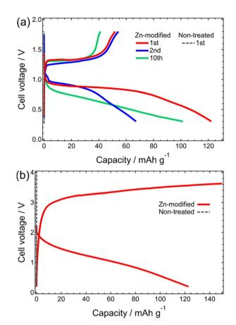
Fig. 4 Discharge-charge profiles of (a) [Zn-modified Mg||Mo<sub>6</sub>S<sub>8</sub>] and (b) [Zn-modified Mg $\|\alpha$ -MnO<sub>2</sub>] cells assembled under a dry-air atmosphere. The profiles using non-modified Mg negative electrodes are included as reference profiles.
