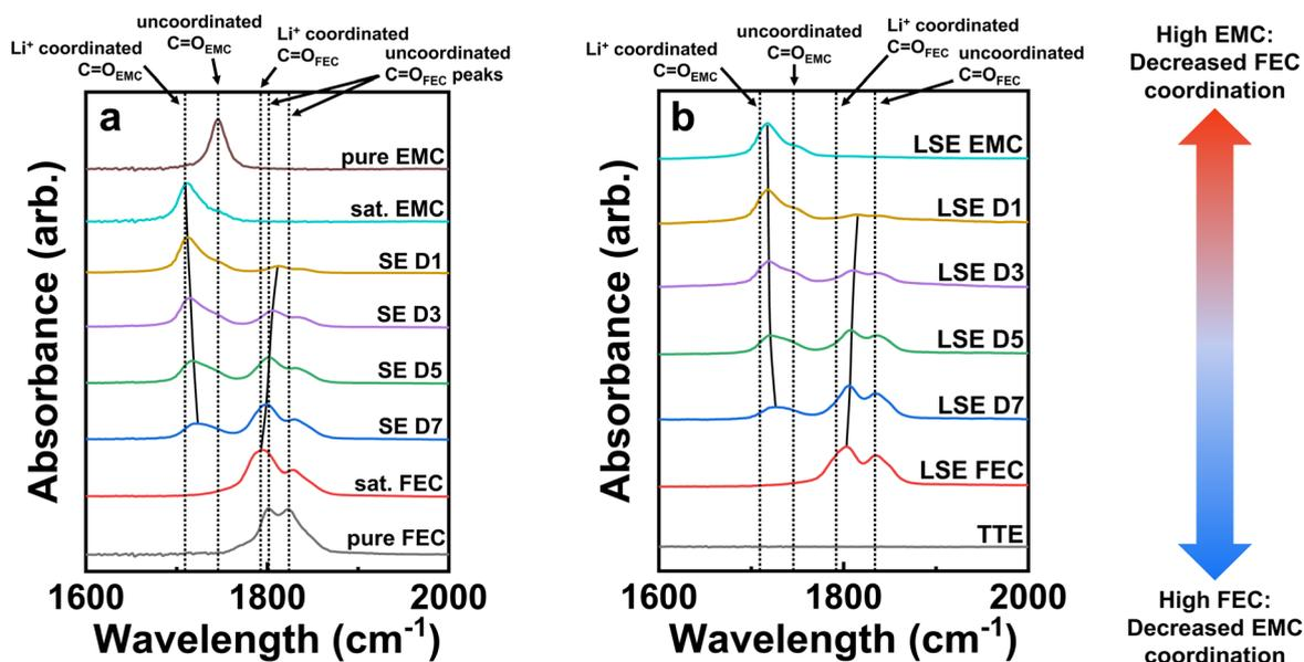
Fig. 6 Characterization of the solvation structures of the various electrolytes. FTIR spectra of the (a) saturated electrolytes along with pure EMC and FEC solvents and (b) LSEs along with pure TTE from 1600 to 2000  $\text{cm}^{-1}$  to study the  $\text{Li}^+$  coordination to solvent molecules. The solid black lines better show the shift in the peak positions with changing FEC to EMC ratios.
