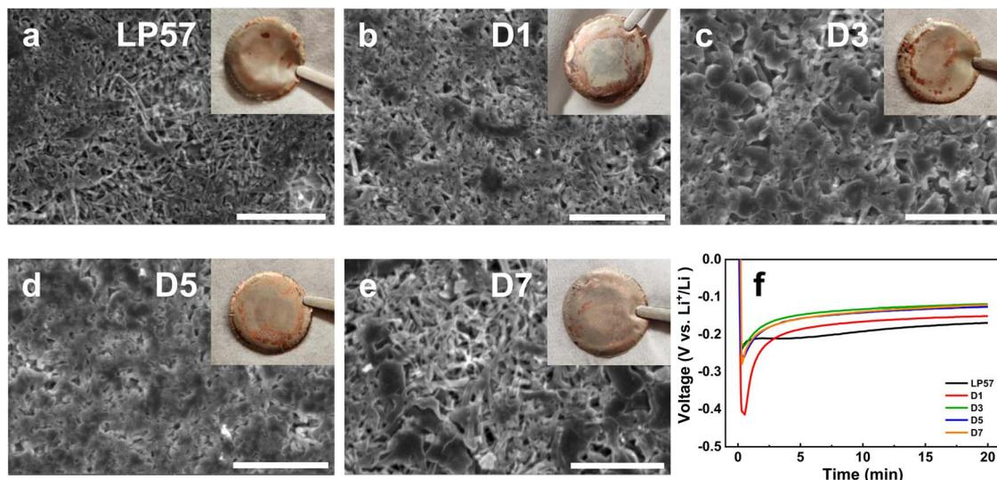
Fig. 4 SEM images of Li plating morphologies on bare Cu foil carried out in Li|Cu cells with (a) LP57, (b) D1, (c) D3, (d) D5, and (e) D7 electrolytes. Insets are photos of the freshly plated Cu foil after cell disassembly. (f) Voltage profiles of the cells during the plating process. A  $1 \text{ mA cm}^{-2}$  current density was applied for 20 minutes for the plating process. All scale bars are  $10 \mu\text{m}$ .
