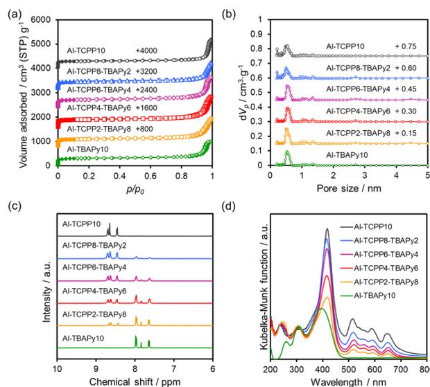
Fig. 3 (a) N<sub>2</sub> physisorption isotherms, (b) pore distributions calculated using NLDFT method, (c) dissolved <sup>1</sup>H-NMR spectra and (d) diffuse-reflectance UV-vis spectra of Al-TCPP(10-X)-TBAPyX samples.
