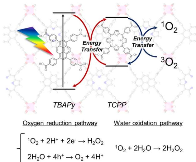
**Scheme 2** Proposed mechanism for photocatalytic  $\text{H}_2\text{O}_2$  production from  $\text{O}_2$  and  $\text{H}_2\text{O}$  over Al-MOFs containing both TBAPy and TCPP linkers via efficient energy transfer.
