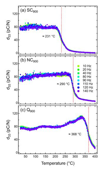
Fig. 11 Temperature-dependent  $d_{33}$  of (a) SC<sub>900</sub>, (b) NC<sub>900</sub>, and (c)  $Q_{900}$  KBT measured between 10 to 140 Hz.
