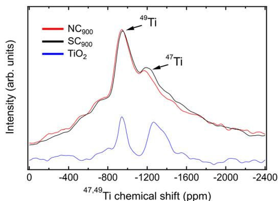
Fig. 7 <sup>47,49</sup>Ti MAS NMR spectra of KBT NC<sub>900</sub> and SC<sub>900</sub>.
