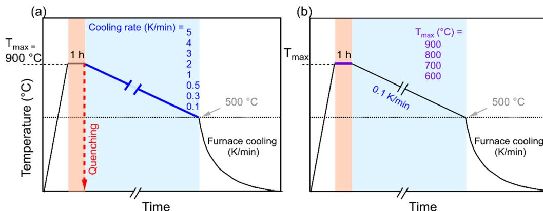
Fig. 1 Annealing profile for KBT as a function of (a) cooling rate from the  $T_{max}$  of 900 °C and (b) different  $T_{max}$  for the cooling rate of 0.1 K min<sup>-1</sup>. The red dashed line in (a) indicates the profile for air quenching from the  $T_{max}$  of 900 °C. In all cases, the heating rate was 5 K min<sup>-1</sup>.
