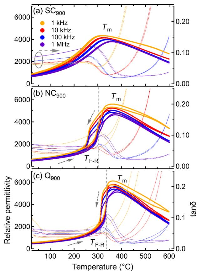
Fig. 4 Variation in temperature-dependent dielectric permittivity and  $\tan\delta$  for (a)  $SC_{900}$ , (b)  $NC_{900}$ , and (c)  $Q_{900}$  KBT ceramics. The vertical dashed line indicates the FE-RE state change temperature,  $T_{\text{F-R}}$  of the  $NC_{900}$  and  $Q_{900}$  KBT.
