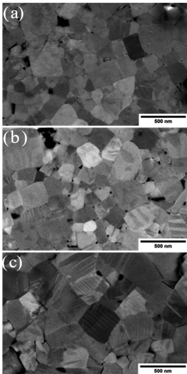
Fig. 8 Microstructure of (a) SC<sub>900</sub>, (b) NC<sub>900</sub>, and (d) Q<sub>900</sub> KBT ceramics.
