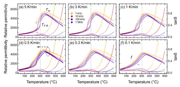
Fig. 2 Variation in temperature-dependent dielectric permittivity and  $\tan \delta$  for KBT ceramics annealed from  $T_{\rm max}$  of 900 °C with different cooling rates (a–f). The vertical line around 304 °C indicates the ferroelectric-relaxor state change temperature  $T_{\rm F-R}$  of the as-processed KBT ceramic is shown for reference.  $T_{\rm m}$  indicates the temperature of maximum permittivity.
