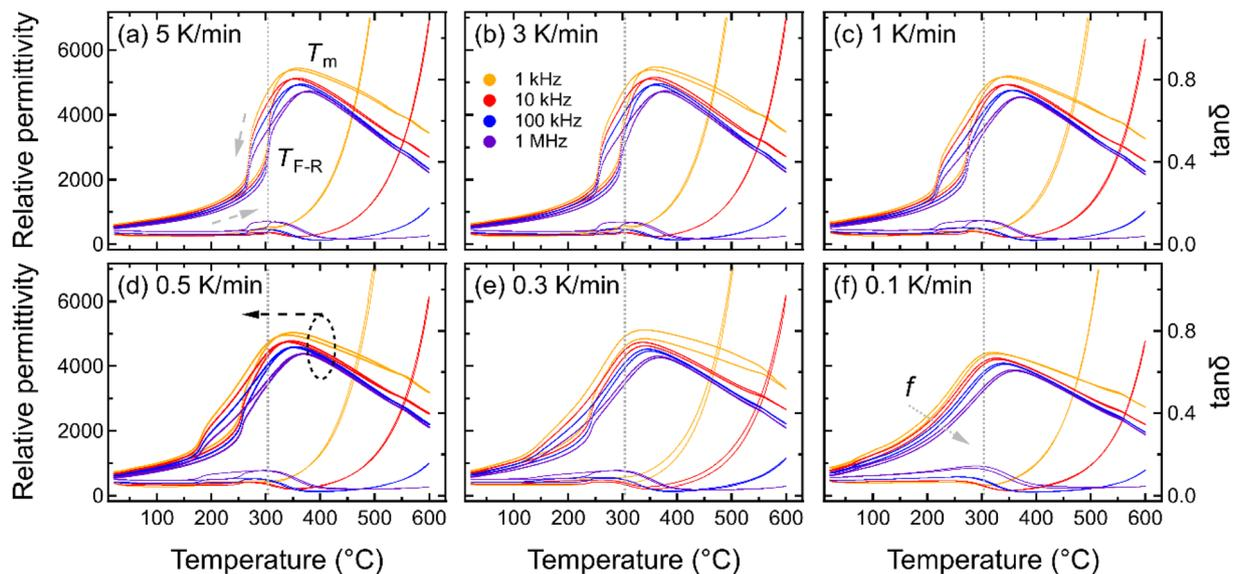
Fig. 2 Variation in temperature-dependent dielectric permittivity and  $\tan \delta$  for KBT ceramics annealed from  $T_{\max}$  of 900 °C with different cooling rates (a–f). The vertical line around 304 °C indicates the ferroelectric-relaxor state change temperature  $T_{F-R}$  of the as-processed KBT ceramic is shown for reference.  $T_m$  indicates the temperature of maximum permittivity.
