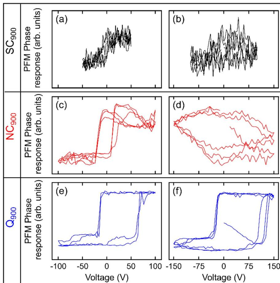
Fig. 10 Local PFM phase hysteresis loops measured at two different spots in (a, b) SC<sub>900</sub>, (c, d) NC<sub>900</sub>, and (e, f) Q<sub>900</sub> KBT ceramics.
