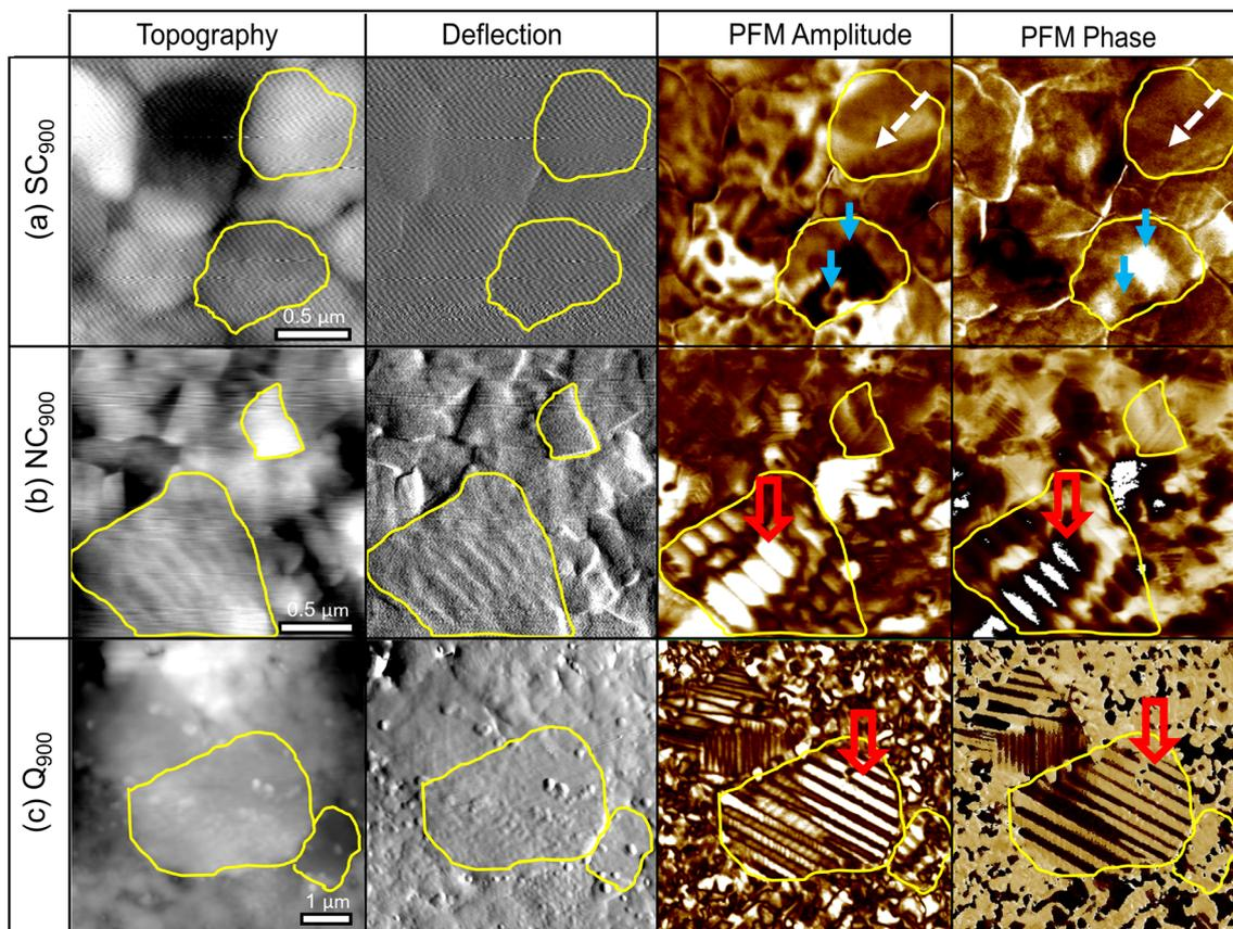
Fig. 9 Topography height and deflection, out-of-plane PFM amplitude and phase images of (a) SC<sub>900</sub>, (b) NC<sub>900</sub>, and (c) Q<sub>900</sub> KBT ceramics. For clarity, two grain boundaries on each panel are marked by a yellow line. An example of grains exhibiting monotonic contrast in the amplitude and phase images is indicated by a dashed white arrow. Examples of regular and irregularly shaped domains are marked by open red and solid blue arrows, respectively.
