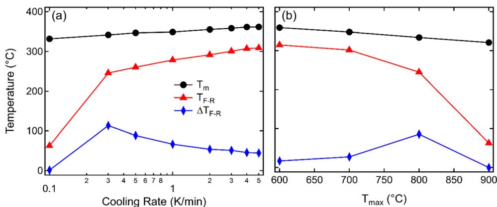
Fig. 3 Variation in  $T_m$ ,  $T_{F-R}$ , and  $\Delta T_{F-R}$  (difference between heating and cooling cycle) depending on (a) the cooling rates from the  $T_{\max}$  of 900 °C and (b) the  $T_{\max}$  of the slowest cooling rate of 0.1 K min<sup>-1</sup>.
