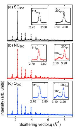
Fig. 5 X-ray diffraction patterns of (a)  $SC_{900}$ , (b)  $NC_{900}$ , and (c)  $Q_{900}$ KBT ceramics measured using bulk-sensitive high-energy XRD. The diffraction patterns are presented as a function of the magnitude of the  $=\frac{4\pi \sin \theta}{}$ scattering vector, q
