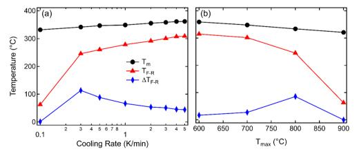
Fig. 3 Variation in  $T_{\rm m}$ ,  $T_{\rm F-R}$ , and  $\Delta T_{\rm F-R}$  (difference between heating and cooling cycle) depending on (a) the cooling rates from the  $T_{\rm max}$  of 900 °C and (b) the  $T_{\rm max}$  of the slowest cooling rate of 0.1 K min<sup>-1</sup>.
