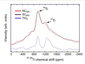
Fig. 7 47,49 Ti MAS NMR spectra of KBT NC<sub>900</sub> and SC<sub>900</sub>.
