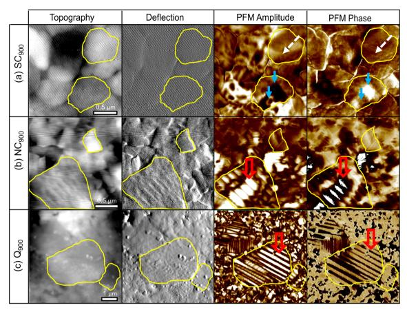
Fig. 9 Topography height and deflection, out-of-plane PFM amplitude and phase images of (a)  $SC_{900}$ , (b)  $NC_{900}$ , and (c)  $Q_{900}$  KBT ceramics. For clarity, two grain boundaries on each panel are marked by a yellow line. An example of grains exhibiting monotonic contrast in the amplitude and phase images is indicated by a dashed white arrow. Examples of regular and irregularly shaped domains are marked by open red and solid blue arrows, respectively.
