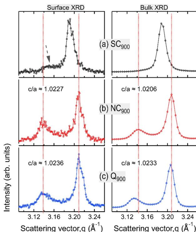
Fig. 6 Variation 002/200 reflections collected from the surface and bulk of (a)  $SC_{900}$ , (b)  $NC_{900}$ , and (c)  $Q_{900}$  KBT. The red vertical lines indicate the position of 002 and 200 reflections of the  $NC_{900}$  sample.
