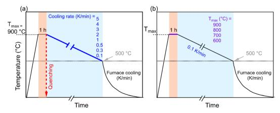
Fig. 1 Annealing profile for KBT as a function of (a) cooling rate from the  $T_{\rm max}$  of 900 °C and (b) different  $T_{\rm max}$  for the cooling rate of 0.1 K min $^{-1}$ . The red dashed line in (a) indicates the profile for air quenching from the  $T_{\rm max}$  of 900 °C. In all cases, the heating rate was 5 K min<sup>-1</sup>.
