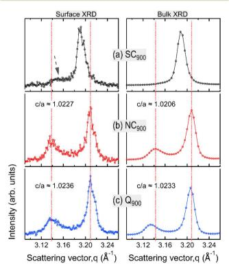
Fig. 6 Variation 002/200 reflections collected from the surface and bulk of (a)  $SC_{900}$ , (b)  $NC_{900}$ , and (c)  $Q_{900}$  KBT. The red vertical lines indicate the position of 002 and 200 reflections of the NC<sub>900</sub> sample.
