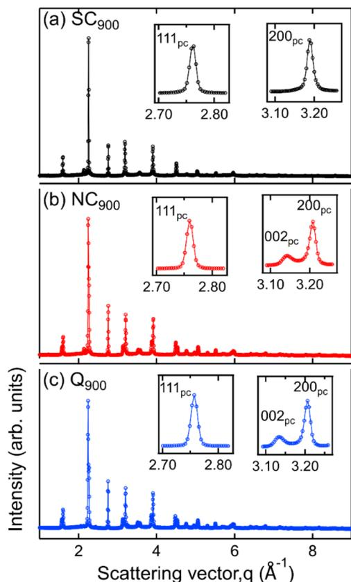
Fig. 5 X-ray diffraction patterns of (a)  $SC_{900}$ , (b)  $NC_{900}$ , and (c)  $Q_{900}$  KBT ceramics measured using bulk-sensitive high-energy XRD. The diffraction patterns are presented as a function of the magnitude of the scattering vector,  $q$  ( $= \frac{4\pi \sin \theta}{\lambda}$ ).
