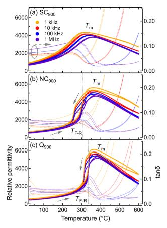
Fig. 4 Variation in temperature-dependent dielectric permittivity and  $\tan\delta$  for (a) SC<sub>900</sub>, (b) NC<sub>900</sub>, and (c) Q<sub>900</sub> KBT ceramics. The vertical dashed line indicates the FE-RE state change temperature,  $T_{\rm F-R}$  of the NC<sub>900</sub> and Q<sub>900</sub> KBT.
