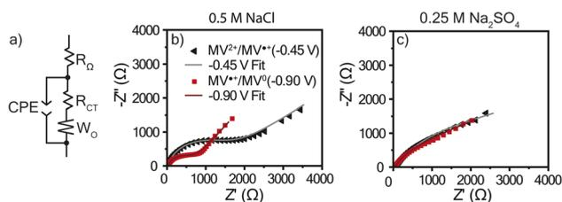
**Fig. 6** (a) The equivalent circuit used to model the EIS data. Nyquist plots for PTPM in (b) 0.5 M NaCl and (c) 0.25 M  $\text{Na}_2\text{SO}_4$  with their curve fits. EIS was conducted at  $-0.45$  V and  $-0.90$  V vs. Ag/AgCl (sat.) with an amplitude of 10 mV in a frequency range of  $5 \times 10^6$  Hz to 0.1 Hz (10 steps per decade). Bode plots are found in Fig. S5 and S6.†
