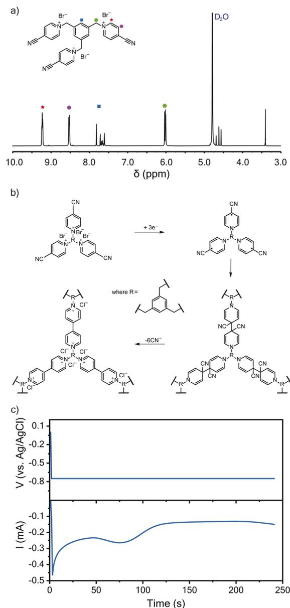
Fig. 1 Synthesis and formation of the crosslinked-viologen network. (a) <sup>1</sup>H-NMR spectra of TPM bromide salt. (b) The electropolymerization mechanism resulting in a crosslinked-viologen network (PTPM). (c) The output current during potentiostatic electropolymerization onto a Au/Ti EQCM-D sensor. The electrolyte was 5 mM TPM in aqueous 0.1 M NaCl. The Au/Ti crystal was the working electrode with a Ag/AgCl reference electrode and platinum plate counter electrode.
