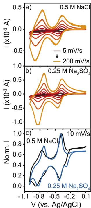
Fig. 2 Cyclic voltammograms at varying scan rates for poly(1,3,5-tris(4-cyanopyridinio)mesitylene) (PTMP) in (a) 0.5 M NaCl and (b) 0.25 M Na<sub>2</sub>SO<sub>4</sub> aqueous electrolyte. (c) Normalized cyclic voltammograms at 10 mV s<sup>-1</sup> for both electrolytes. PTMP electropolymerized on the Au/Ti EQCM-D crystal was the working electrode with a Ag/AgCl reference electrode and platinum plate counter electrode. The legend in (a) applies to (b).
