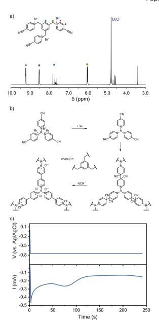
Fig. 1 Synthesis and formation of the crosslinked-viologen network. (a) <sup>1</sup>H-NMR spectra of TPM bromide salt. (b) The electropolymerization mechanism resulting in a crosslinked-viologen network (PTPM). (c) The output current during potentiostatic electropolymerization onto a Au/Ti EQCM-D sensor. The electrolyte was 5 mM TPM in aqueous 0.1 M NaCl. The Au/Ti crystal was the working electrode with a Ag/AgCl reference electrode and platinum plate counter electrode.
