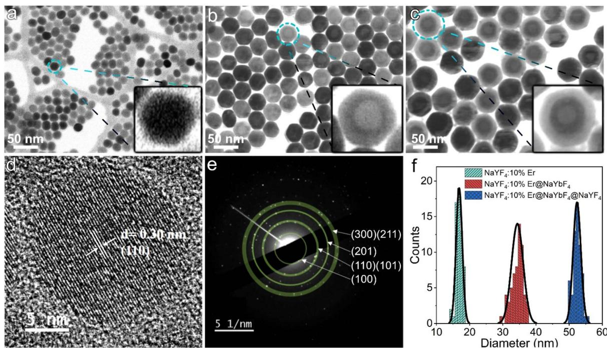
Fig. 2 SEM images of (a) NaYF<sub>4</sub>:10%Er core, (b) NaYF<sub>4</sub>:10%Er@NaYbF<sub>4</sub> core-shell, and (c) NaYF<sub>4</sub>:10%Er@NaYbF<sub>4</sub>@NaYF<sub>4</sub> core-shell-shell. (d) HRTEM image of a single NaYF<sub>4</sub>:10%Er core and (e) the corresponding SAED pattern. (f) Particle size statistics based on SEM images.
