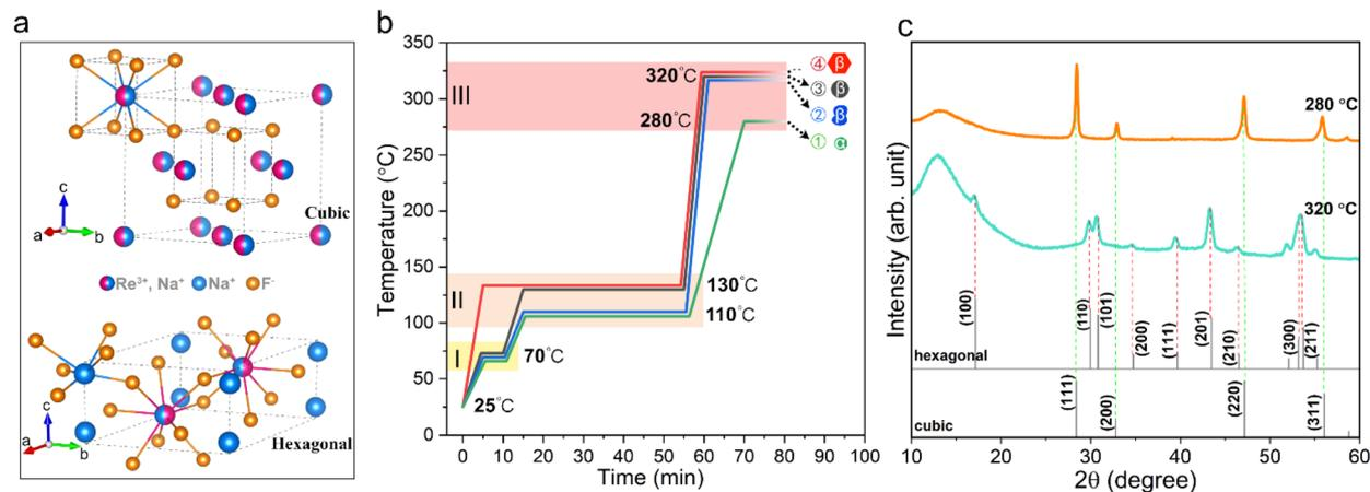
Fig. 1 (a) Schematic diagram of the crystal structure of cubic and hexagonal NaYF<sub>4</sub>. (b) Temperature profiles used for synthesizing UCNPs during the thermal decomposition process. (c) XRD patterns of NaYF<sub>4</sub> nanoparticles synthesized at growth temperatures of 280 °C and 320 °C.
