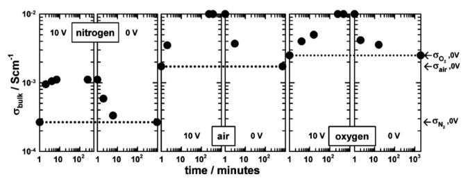
Fig. 3 Bulk conductivity of BaTi<sub>0.99</sub>Ca<sub>0.01</sub>O<sub>2.99</sub> with 10 V bias in different atmospheres at 600 °C; reproduced from N. Maso *et al.*, *Appl. Phys. Lett.*, 2010, **97**, 062907 with permission from AIP publishing.
