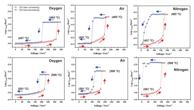
Fig. 9 Total conductivity at two temperatures and in atmospheres of different  $pO_2$  of  $Hf_{0.85}Y_{0.15}O_{1.925}$  on a stepwise cycle of increasing and decreasing applied voltage after reaching a steady state at each voltage; reproduced from ref. 12: M. Alotaibi *et al.*, *J. Am. Ceram. Soc.*, 2023, **106**, 822 with permission from Wiley publishing.
