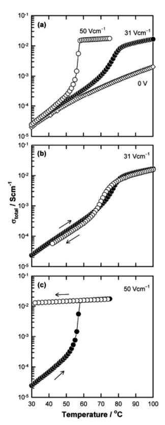
Fig. 7 Bulk conductivity of  $Bi_{0.95}Ca_{0.05}FeO_3$  against temperature without and with applied fields of 31 and 50 V cm<sup>-1</sup>; reproduced from N. Maso *et al.*, *Phys. Chem. Chem. Phys.*, 2014, **16**, 19408 with permission from the PCCP owner societies.
