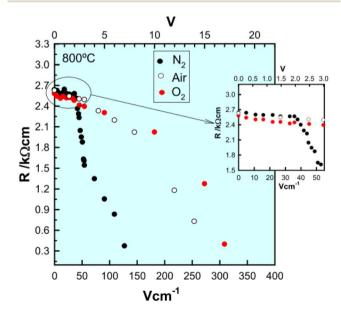
Fig. 5 Resistance of  $Y_{0.5}Zr_{0.49}Mg_{0.01}O_{1.74}$  as a function of bias voltage at 800 °C in different atmospheres; reproduced from M. Jovani et al., Sci. Rep., 2019, 9, 18538, with permission from Springer Nature.
