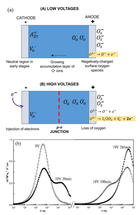
Fig. 6 (a) Model for voltage-dependent resistance at low and higher voltages; reproduced from M. Jovani et al., Sci. Rep., 2019, **9**, 18538 with permission from Springer Nature; (b) M'' spectra showing evolution with time of the electrical microstructure of BaTi<sub>0.99</sub>Mg<sub>0.01</sub>O<sub>2.99</sub> ceramic with a bias voltage of 10 V at 242 °C; reproduced from M. Prades et al., J. Mater. Chem., 2010, **20**, 5335 with permission from the Royal Society of Chemistry.
