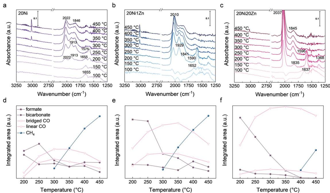
Fig. 4 *In situ* DRIFTS spectra of (a) 20Ni, (b) 20Ni1Zn, and (c) 20Ni20Zn during CO<sub>2</sub> hydrogenation. Evolution of species in *in situ* DRIFTS of (d) 20Ni, (e) 20Ni1Zn, and (f) 20Ni20Zn.
