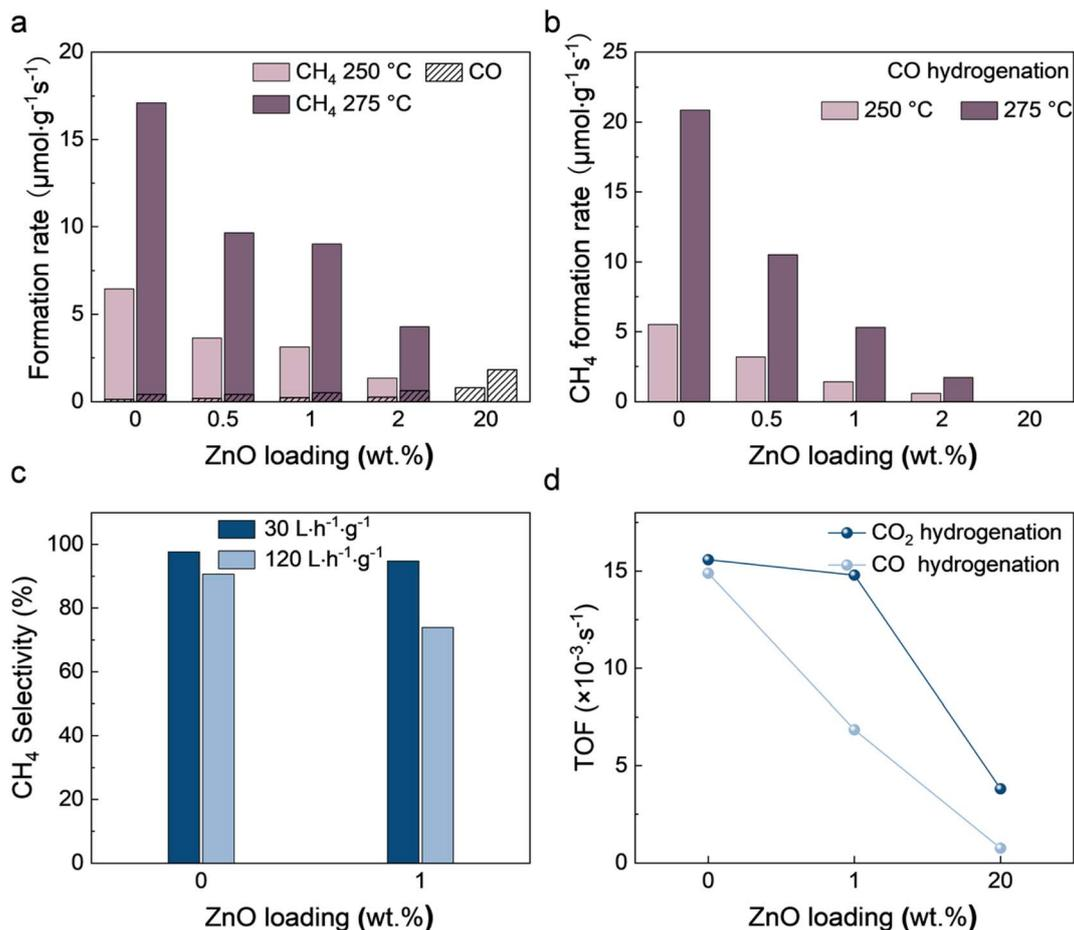
Fig. 1 Catalytic performance of (a) CO<sub>2</sub> and (b) CO hydrogenation, (c) space velocity dependency evaluation results, and (d) TOF of NiZn/Al<sub>2</sub>O<sub>3</sub> catalysts.
