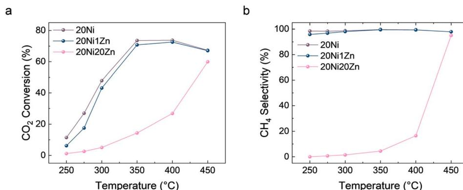
Fig. 5 CO<sub>2</sub> hydrogenation activity of NiZn/Al<sub>2</sub>O<sub>3</sub> catalysts over a wider range of temperatures.
