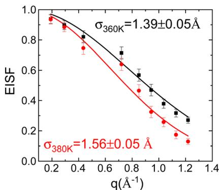
Fig. 4 Elastic incoherent structure factor obtained for HQuin as a sum of momentum transfer for the two measured temperatures ( $T = 380$  K red circles,  $T = 360$  K black squares). Solid lines are fits of the experimental data to eqn (2).
