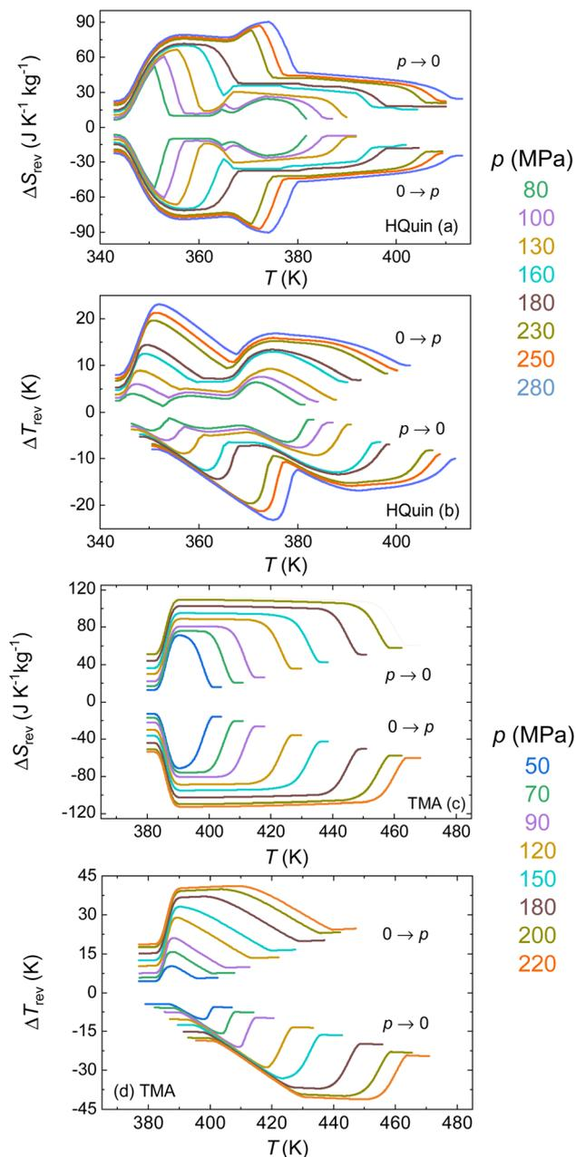
**Fig. 9** Reversible isothermal entropy changes on decompression and compression as a function of temperature at different pressures for HQuin (a) and TMA (c). Reversible adiabatic temperature changes on decompression and compression as a function of temperature at different pressures for HQuin (b) and TMA (d).
