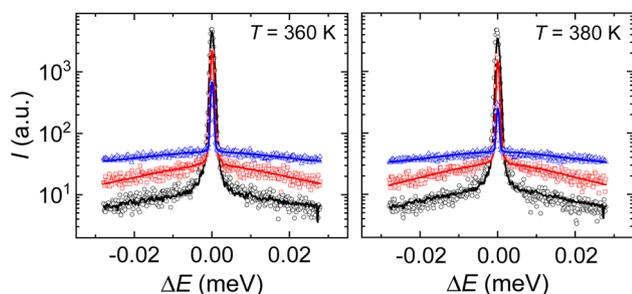
Fig. 3 Representative experimental neutron scattering spectra of HQuin for selected momentum transfer (symbols) ( $q_1 = 0.29 \text{ \AA}$ : black circles,  $q_2 = 0.85 \text{ \AA}$ : red squares,  $q_3 = 1.22 \text{ \AA}$ : blue triangles). The spectrum at momentum transfer  $q_3$  has been shifted upwards by 20 units. Lines show the fittings using eqn (1).
