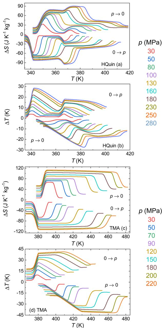
**Fig. 8** Barocaloric effects obtained on first application or removal of pressure. Isothermal entropy changes on decompression and compression as a function of temperature at different pressures for HQuin (a) and TMA (c). Adiabatic temperature changes on decompression and compression as a function of temperature at different pressures for HQuin (b) and TMA (d).
