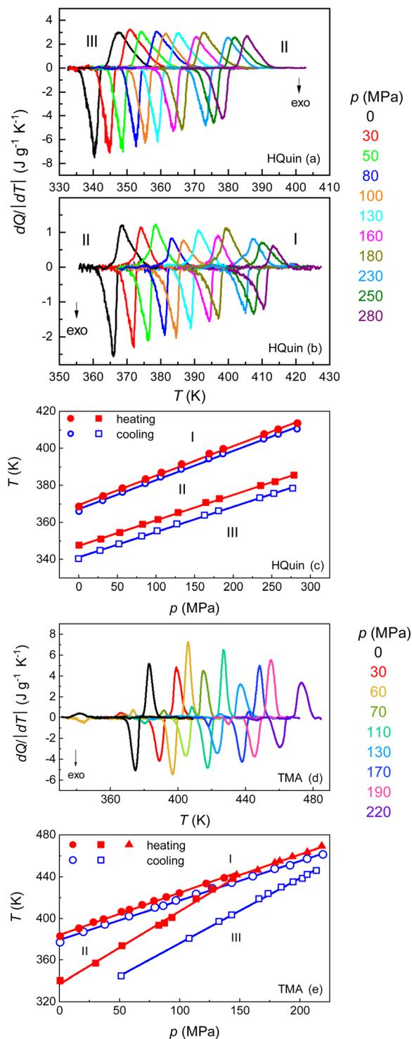
Fig. 6 Temperature-dependent isobaric heat flow  $dQ/dT$  at different pressures, after baseline subtraction for HQuin (a,b) and TMA (d). Peak temperature across the phase transition as a function of pressure determined from both heating and cooling heat flow curves for HQuin (c) and TMA (e).
