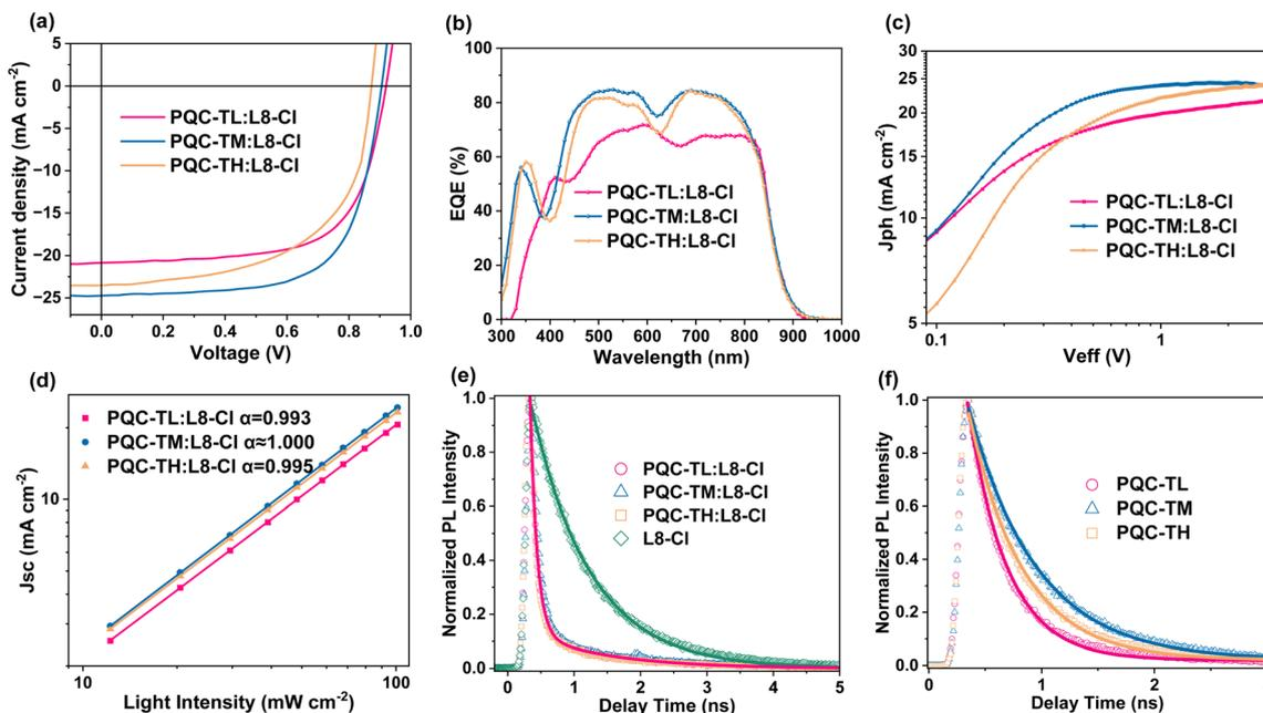
Fig. 2 (a) *J-V* characteristics, (b) EQE curves, (c) *J<sub>ph</sub>*-*V<sub>eff</sub>* curves, and (d) dependence of current density on light intensity of the OPVs based on PQC-TL:L8-Cl, PQC-TM:L8-Cl and PQC-TH:L8-Cl. (e) Time-resolved photoluminescence (TRPL) decay kinetics of PQC-TL:L8-Cl, PQC-TM:L8-Cl, PQC-TH:L8-Cl and L8-Cl films excited at 550 nm. (f) TRPL decay kinetics of PQC-TL, PQC-TM, and PQC-TH neat films excited at 550 nm.
