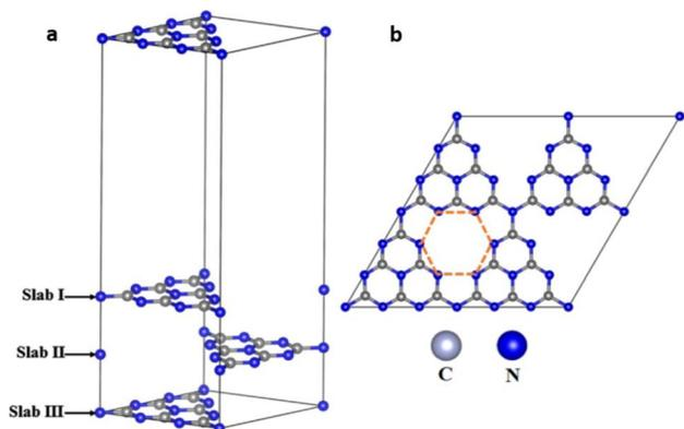
Fig. 12 (a) Schematic representation of three-layer  $g\text{-C}_3\text{N}_4$  model, (b)  $2 \times 2 \times 1$  supercell monolayer  $g\text{-C}_3\text{N}_4$ . The highlighted ring composed of six numbers of bi-coordinated nitrogen atoms is referred to as six-fold cavity. Reproduced with permission from ref. 7. Copyright 2018 Elsevier.
