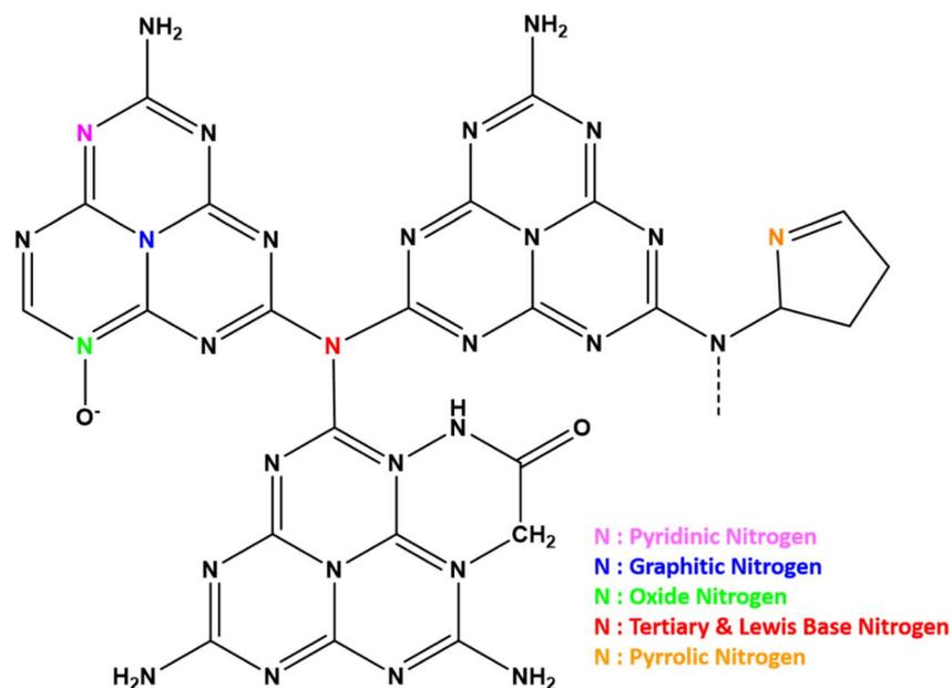
Fig. 3 Types of nitrogen functionalities possible in  $g\text{-C}_3\text{N}_4$ .
