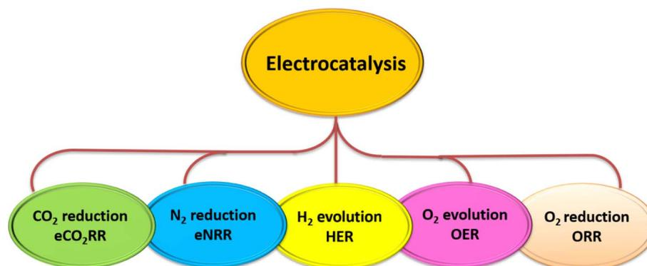
Fig. 29 Various electrocatalytic reactions catalysing by g-C<sub>3</sub>N<sub>4</sub> based SACs.
