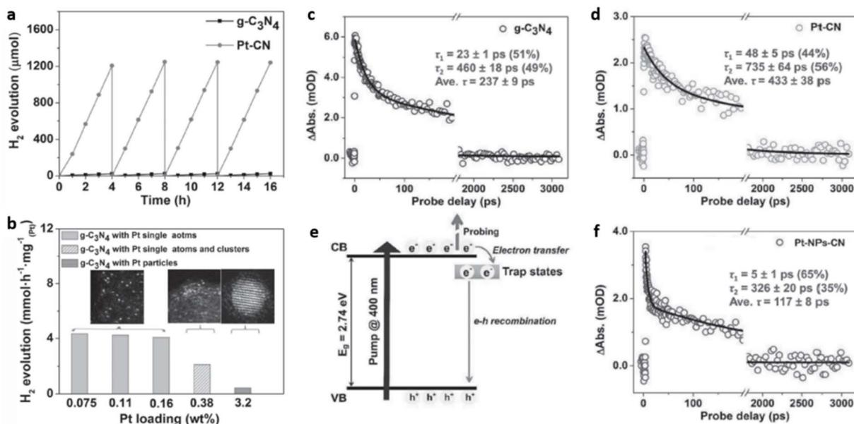
Fig. 16 (a) Photocatalytic H<sub>2</sub> evolution with time for g-C<sub>3</sub>N<sub>4</sub> and Pt-CN, (b) photocatalytic H<sub>2</sub> evolution with varying Pt content (normalised per Pt atom), average recovery life time values in mOD (optical density) of (c) g-C<sub>3</sub>N<sub>4</sub>, (d) Pt-CN, (e) an illustration of the various mechanisms involved, (f) data on TA kinetics for Pt-NPs-CN. Reproduced with permission from ref. 64. Copyright 2016 John Wiley and Sons.
