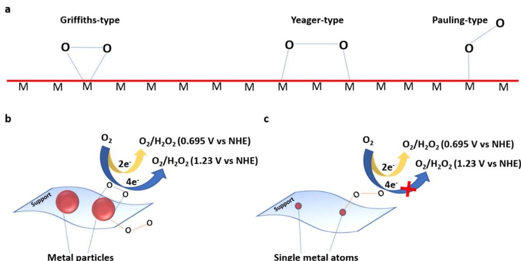
Fig. 23 (a) O<sub>2</sub> adsorption modes on a metal surface, ORR pathways on (b) metal nanoparticles and (c) single metal atom sites.
