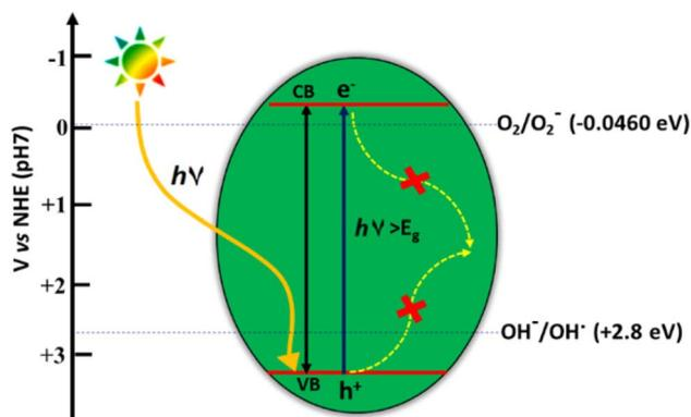
Fig. 21 Schematic of the photocatalytic process.
