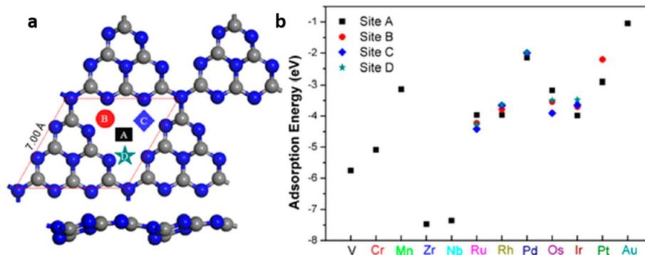
Fig. 27 (a) Possible adsorption sites for single metal atoms in  $\text{g-C}_3\text{N}_4$  layer, (b) adsorption energies of various metal single atoms on available adsorption sites in the  $\text{g-C}_3\text{N}_4$  surface. Reproduced with permission from ref. 115. Copyright 2020 American Chemical Society.
