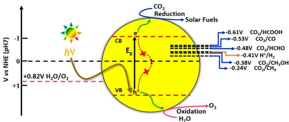
Fig. 13 Schematic illustration of photocatalytic carbon dioxide reduction.
