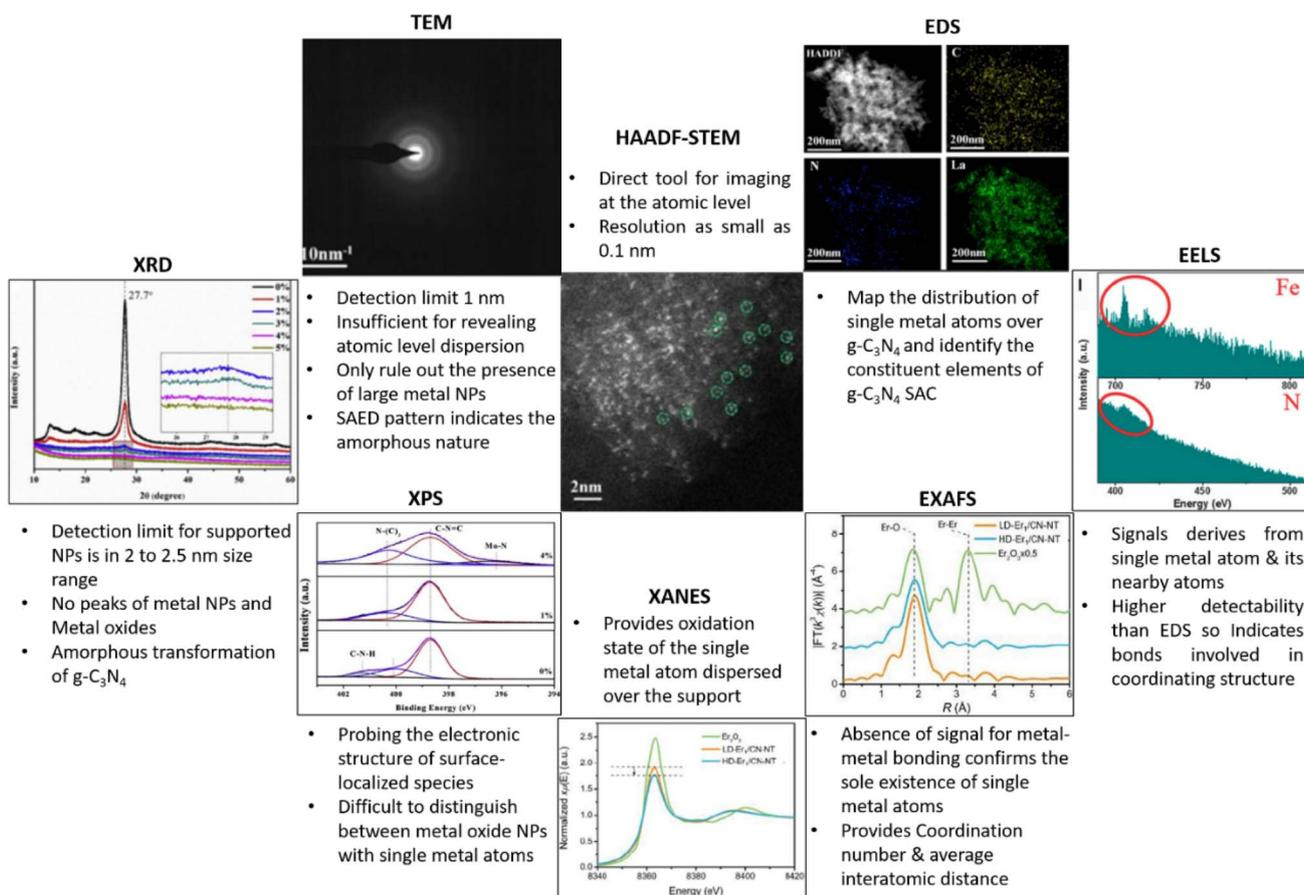
Fig. 8 Various analytical tools for the characterisation  $g\text{-C}_3\text{N}_4$  based SACs. Reproduced with permission from ref. 9. Copyright 2020 John Wiley and Sons. Reproduced with permission from ref. 16. Copyright 2020 American Chemical Society. Reproduced with permission from ref. 27. Copyright 2019 Elsevier. Reproduced from ref. 28.
