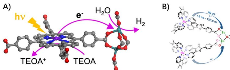
Fig. 5 (A) The ligand-to-node multielectron transfer from excited porphyrin-linkers to Ru<sub>2</sub> SBUs. Reprinted with permission from ref. 30. Copyright 2018 American Chemical Society. (B) Schematic light-induced electron transfer from Ru-metalloligand photocenter to catalytic Eu<sub>2</sub> oxo-cluster center in Eu-Ru(phen)<sub>3</sub>-MOF. Reprinted from ref. 64.
