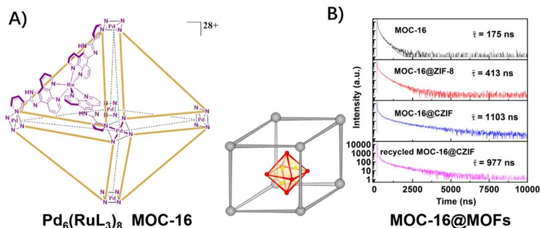
Fig. 9 (A) The structure of a PMD of the Pd<sub>6</sub>(RuL<sub>3</sub>)<sub>8</sub> metal-organic cage (MOC-16); (B) time-resolved emission decay of the <sup>3</sup>MLCT excited-state of MOC-16 and MOC-16@MOFs. Reprinted with permission from ref. 49. Copyright 2019 American Chemical Society.
