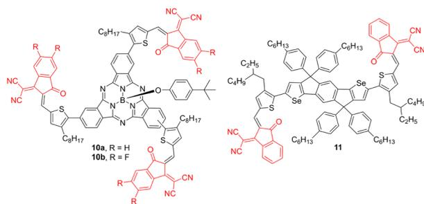
Fig. 5 The molecular structures of subphthalocyanine and thiophene-selenophene cores decorated with IC acceptor.
