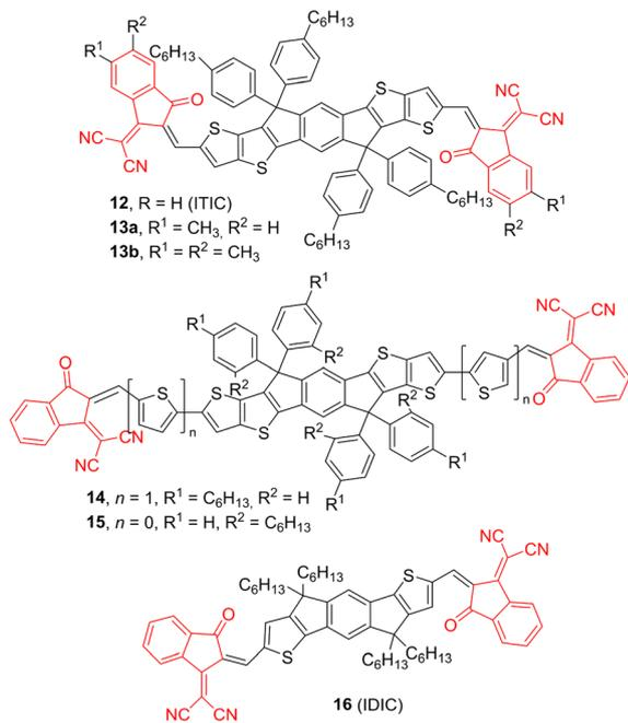
Fig. 6 ITIC family of small acceptors for OSCs.
