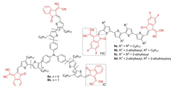
Fig. 4 The molecular structures of TPA (**8**)- and oligothiophene (**9**)-based semiconductors bearing peripheral IC and FIC acceptors.
